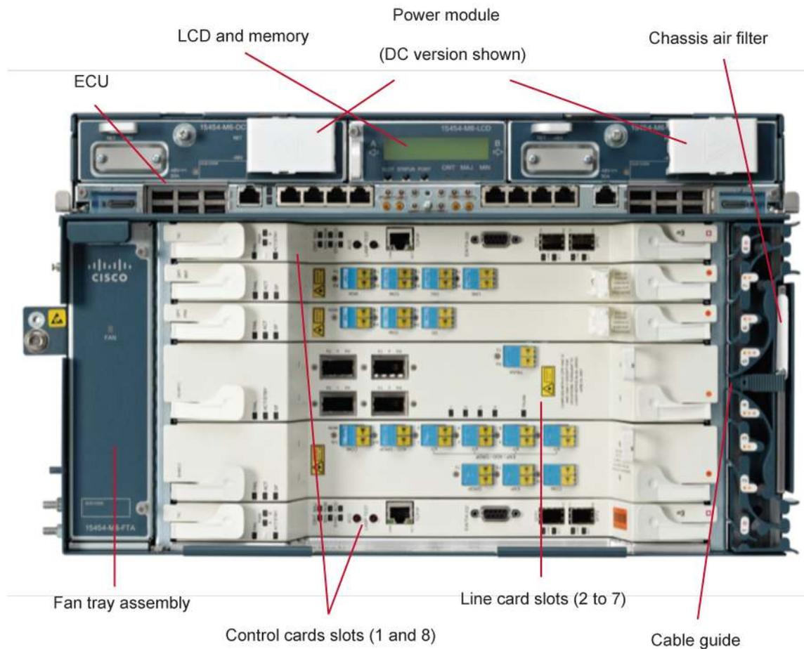
**Figure 3.** Electrical Connection Unit (ECU)
