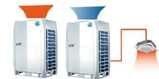
Stage 1: Operation in continuous heating mode
