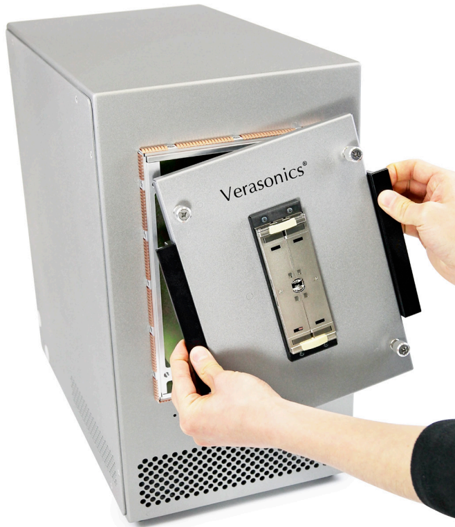
The UTA can be changed in about one minute — no tools required
