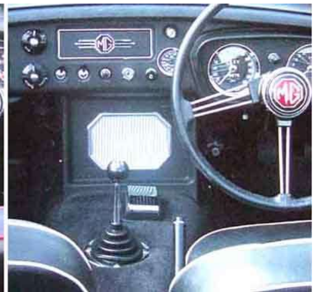
A 73 cranked to the right to clear the tunnel console, changing at chassis number 258001 for the 1972 model year, albeit on an LHD: (Clausager)
