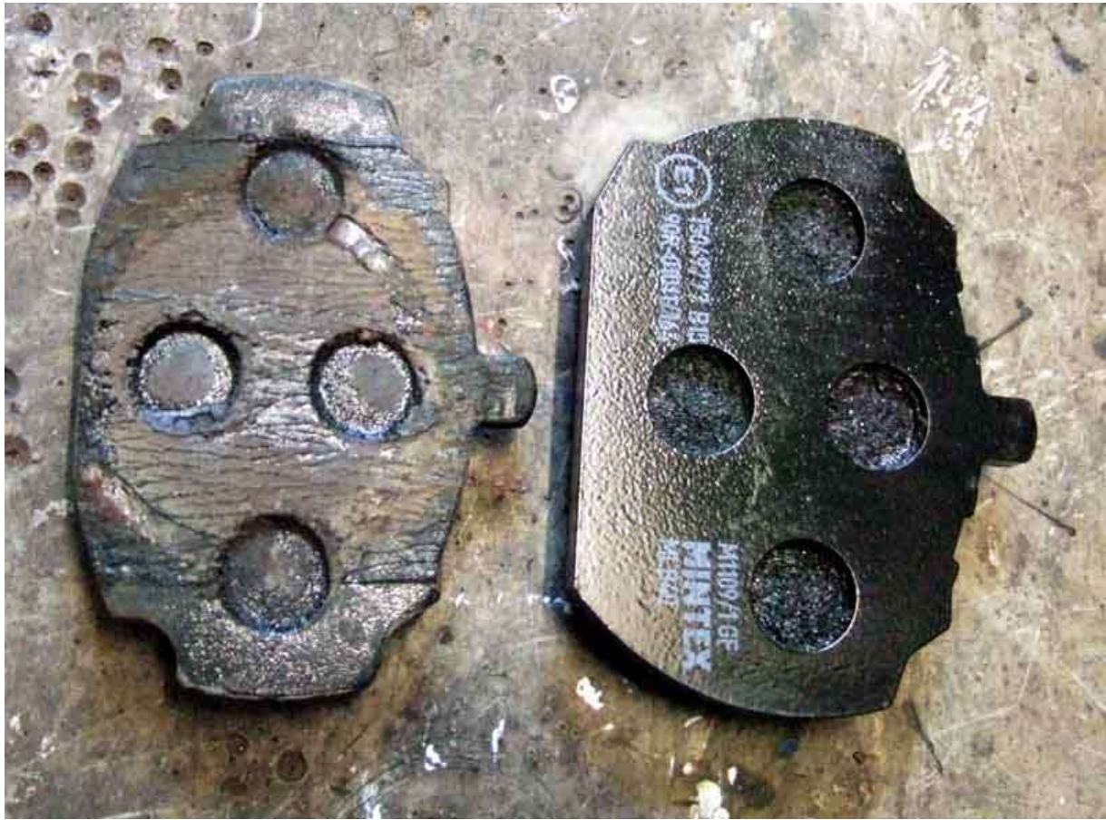
V8 pads in 4-cylinder calipers: With the 'tops' aligned the 'bottoms' of the V8 pads extend a bit further:
