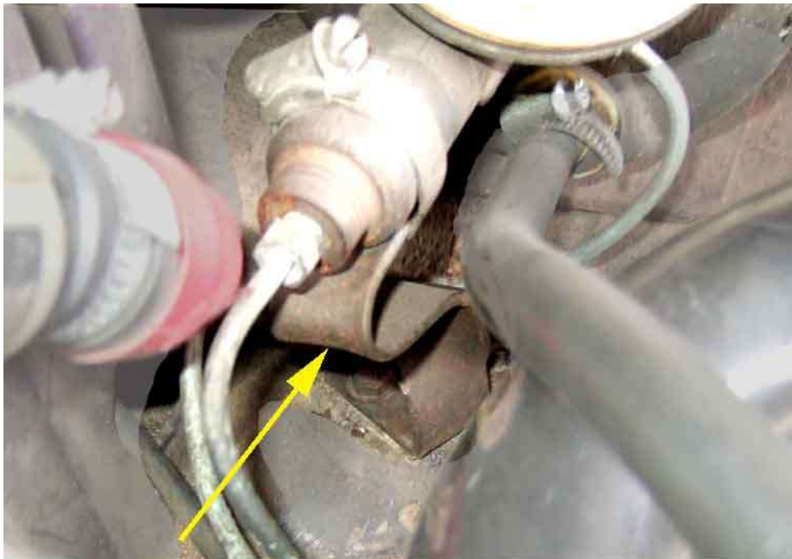
Cylinder support - a crude 'S'-shape secured to the servo with a Jubilee clip:
