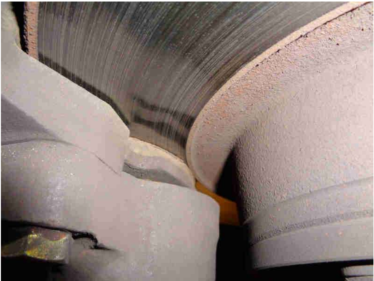
V8 pad with 4-cylinder caliper and disc:
