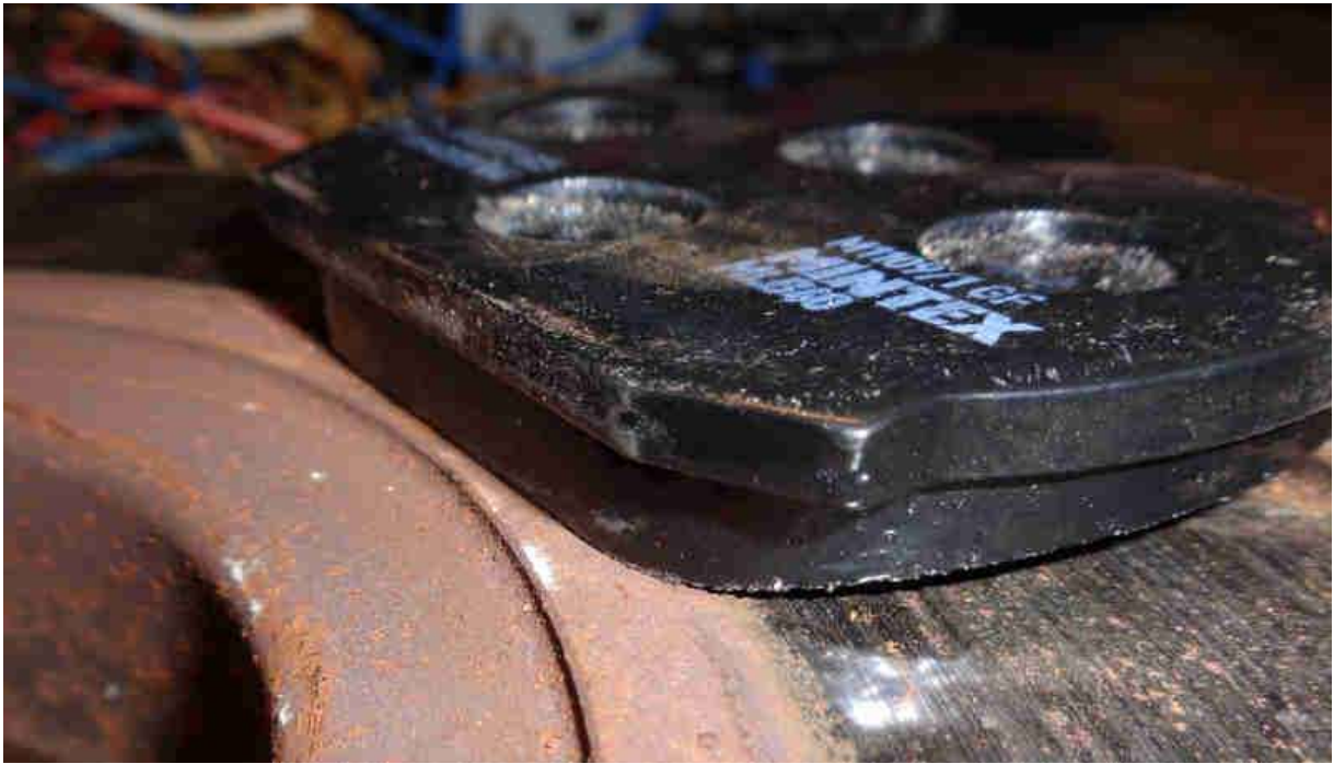
Confirmed in the caliper - 4-cylinder pad with 4-cylinder caliper and disc:
