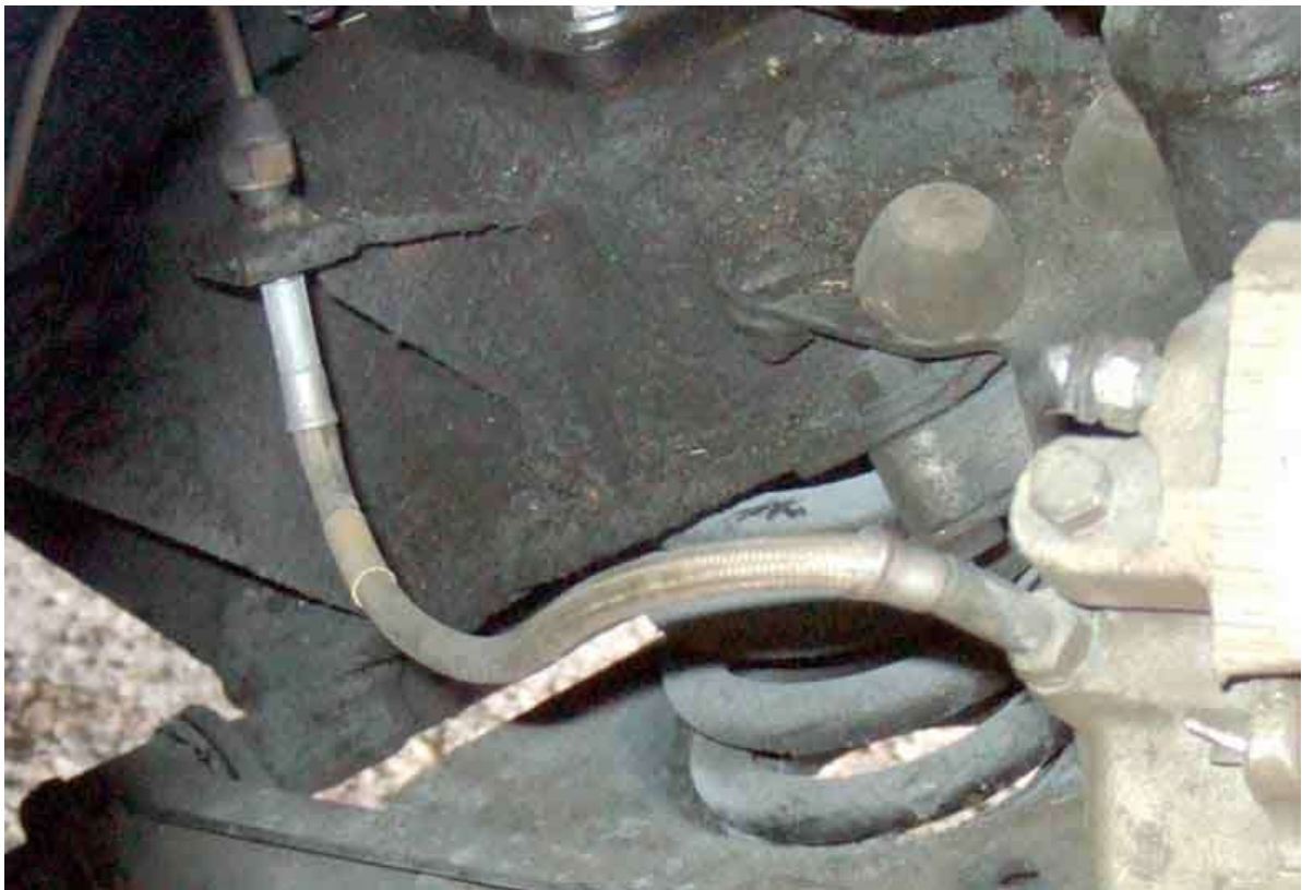
Vee's, with 330mm from hex face to hex face, but with 33mm metal ends:
