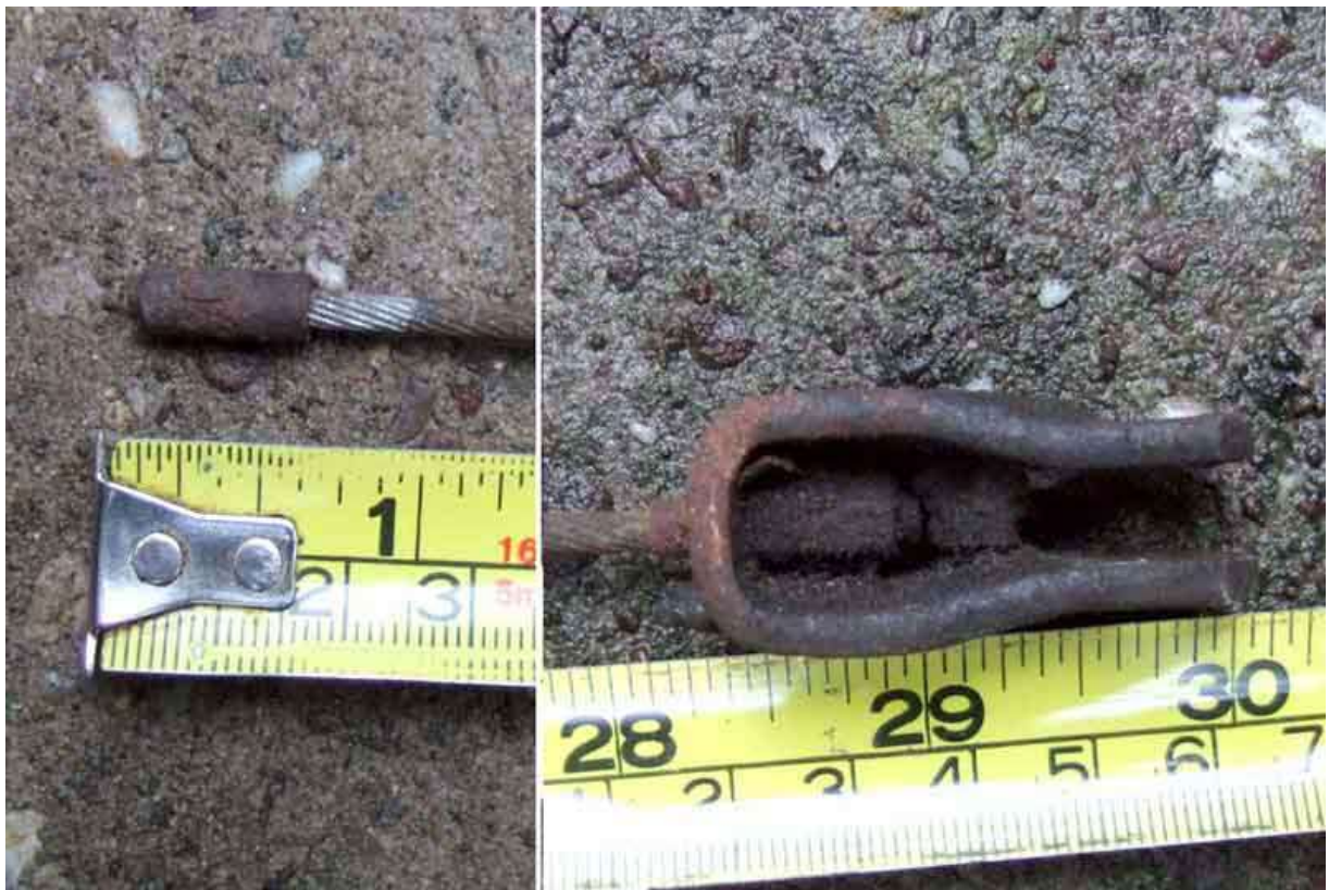
A 1" 'shortener' fitted between the nipple and the fitting on the end of the outer sheath at the compensation lever
