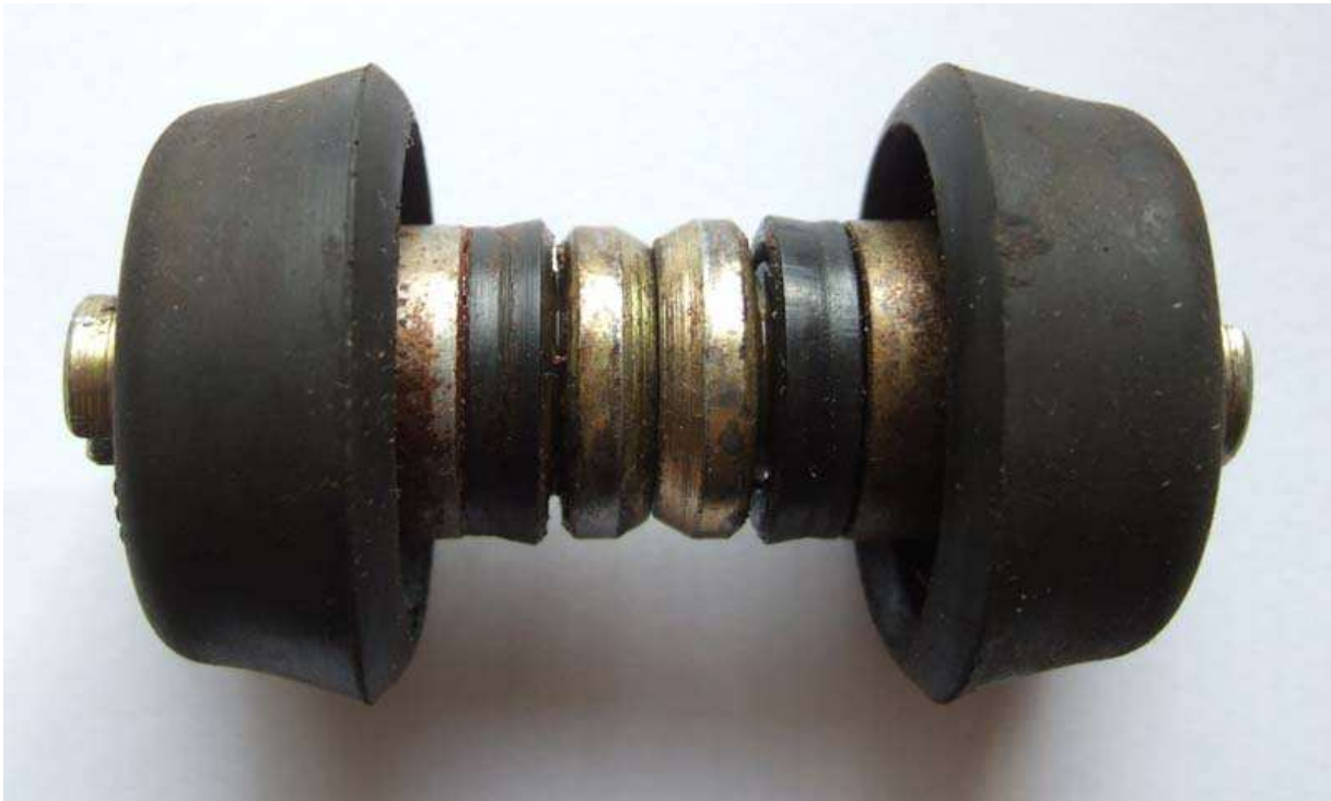
2021 and Vee's off-side wheel cylinder. Outside shiny metal but very rusty under the cover, as are the piston and bore outside the seals:
