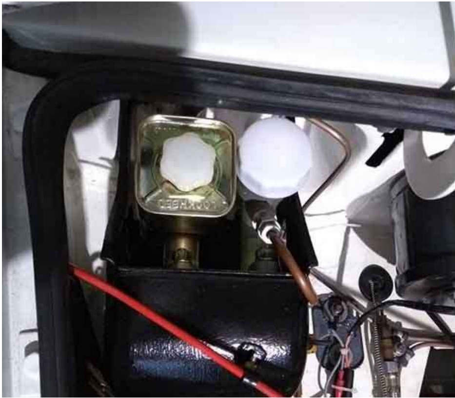
The 'ink' is hardly dry on the above and Ray has fitted a Girling brake master:
