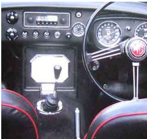
A 73 cranked to the right to clear the tunnel console, changing at chassis number 258001 for the 1972 model year, albeit on an LHD: (Clausager)
