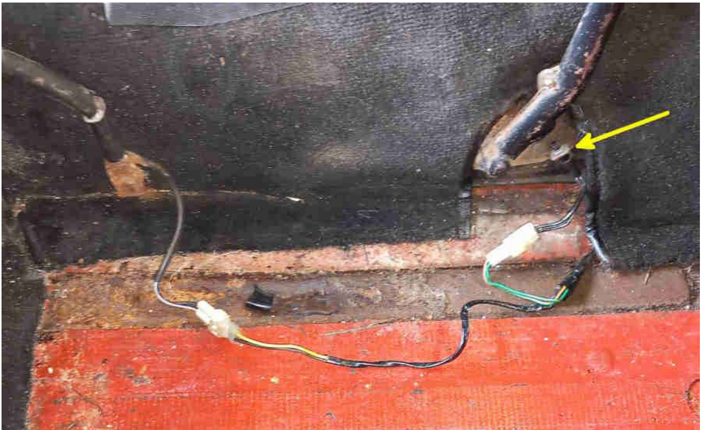
The handbrake switch used is AAU2492: ( Brown & Gammons )
