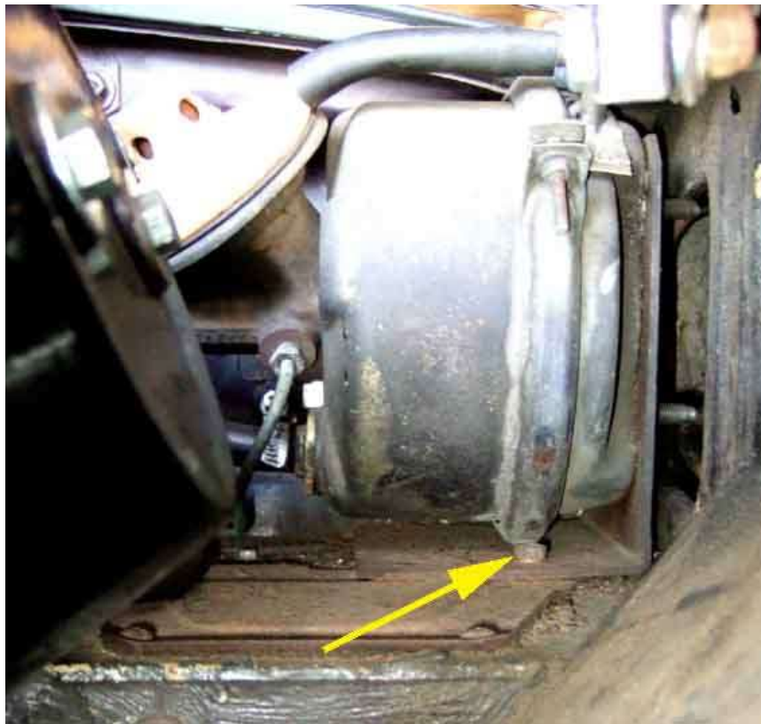
Cylinder support - a crude 'S'-shape secured to the servo with a Jubilee clip:
