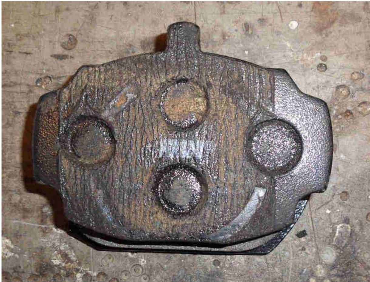
There is noticeably more friction material closer to the stub-axle:
