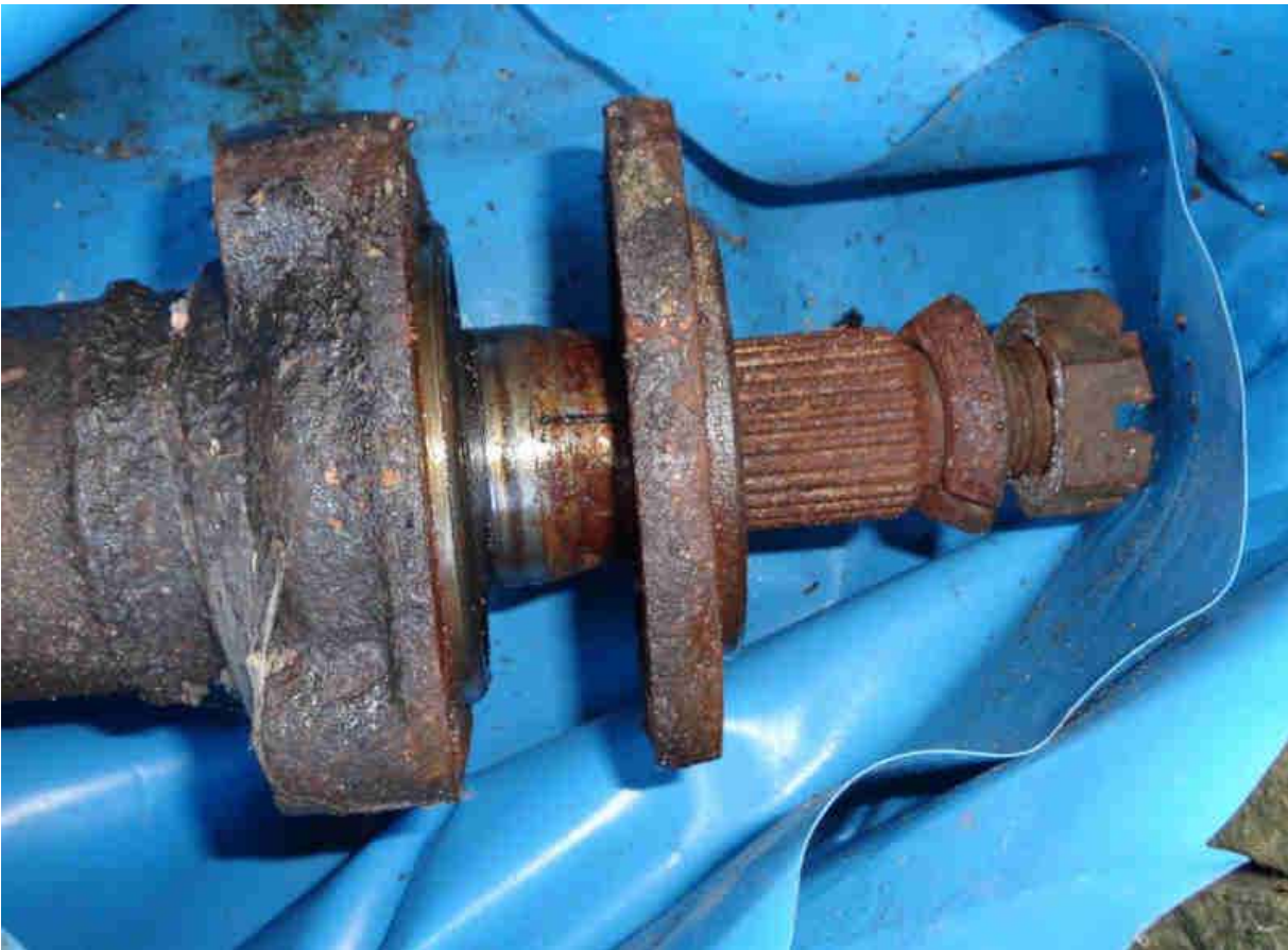
Father Ted's half-shaft with a clear gap between spacer and shaft shoulder:
