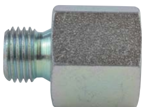
B.21.0089 NIPPLES 1/4" BSP FEMALE - 7/16" UNF MALE
