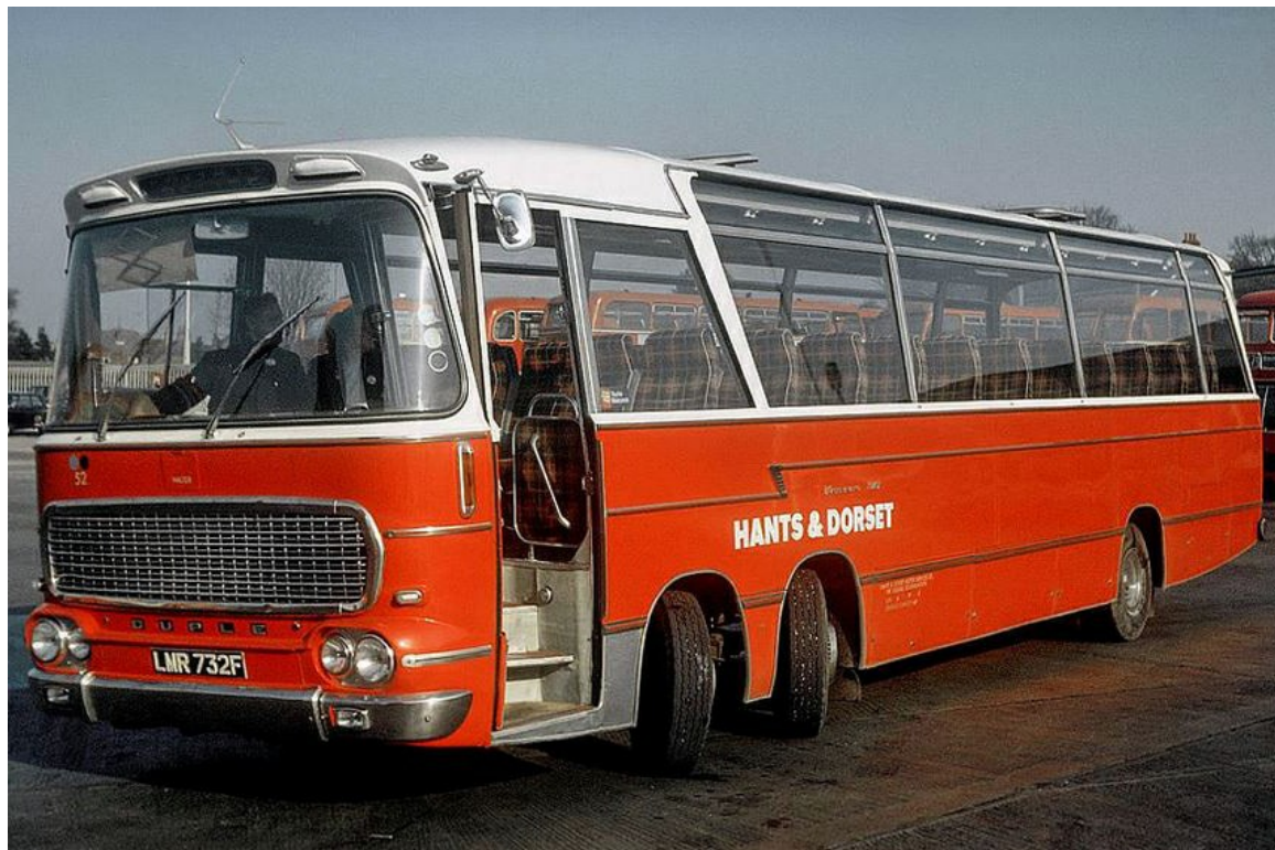
No. 52 (LMR732F) was a Duple 49-seat coach bodied Bedford VAL70 that was among the vehicles absorbed into the Hants & Dorset fleet from Wilts & Dorset in 1972. (LTHL collection).
