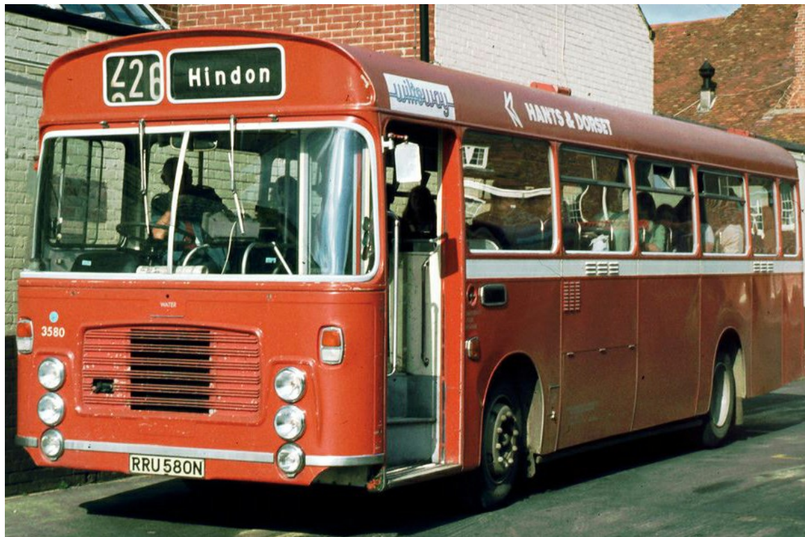
No. 3580 (RRU580N) was a very 'Bristol' looking Ford R1014 with ECW 45-seat bodywork. It was withdrawn in 1981. (Clive Brown).
