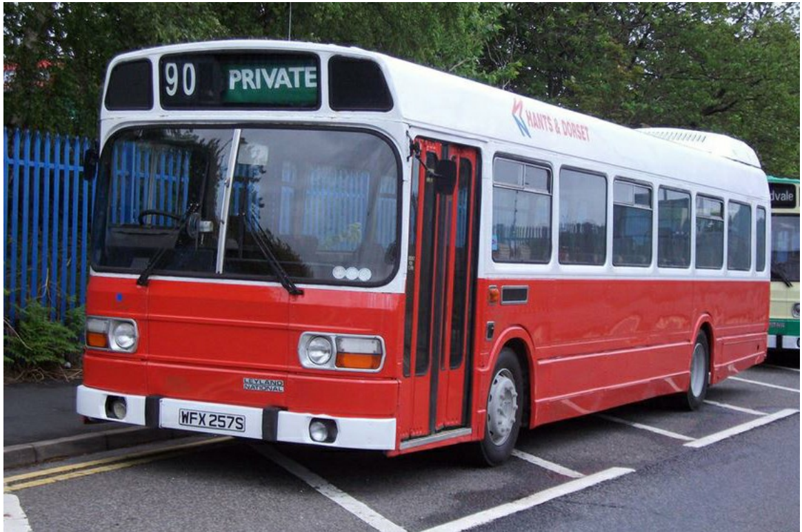
No. 3732 (WFX257S), a 1978 Leyland National with 48-seat dual purpose bodywork. It was one of the vehicles that passed to the Provincial Bus Company in 1983 on the break up of Hants & Dorset. (Trevor Harrison).
