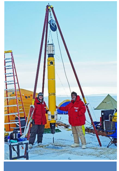
GA Tech used a 3.5 mm Linden STFOC tether on a NASA funded project to deploy a 10 ft long ROV the under Ross Ice Shelf in Antarctica capturing never before seen footage.
