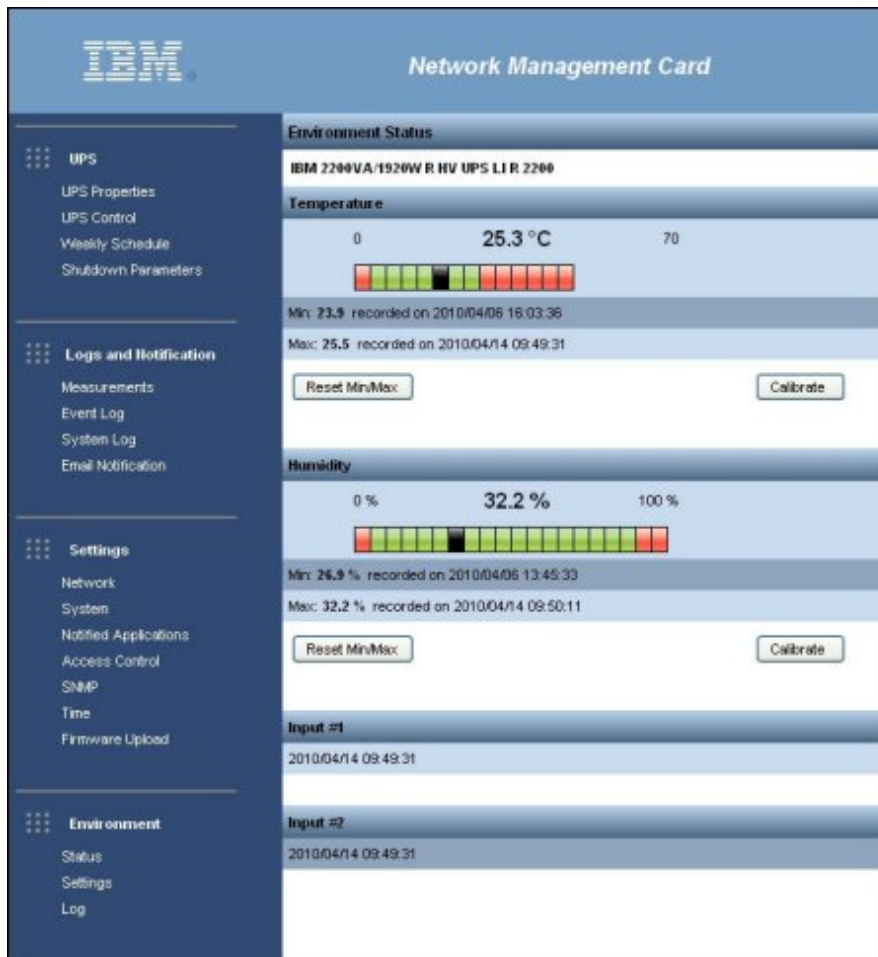
Figure 13. Environmental Monitoring Probe data as viewed from the Network Management Card web interface
