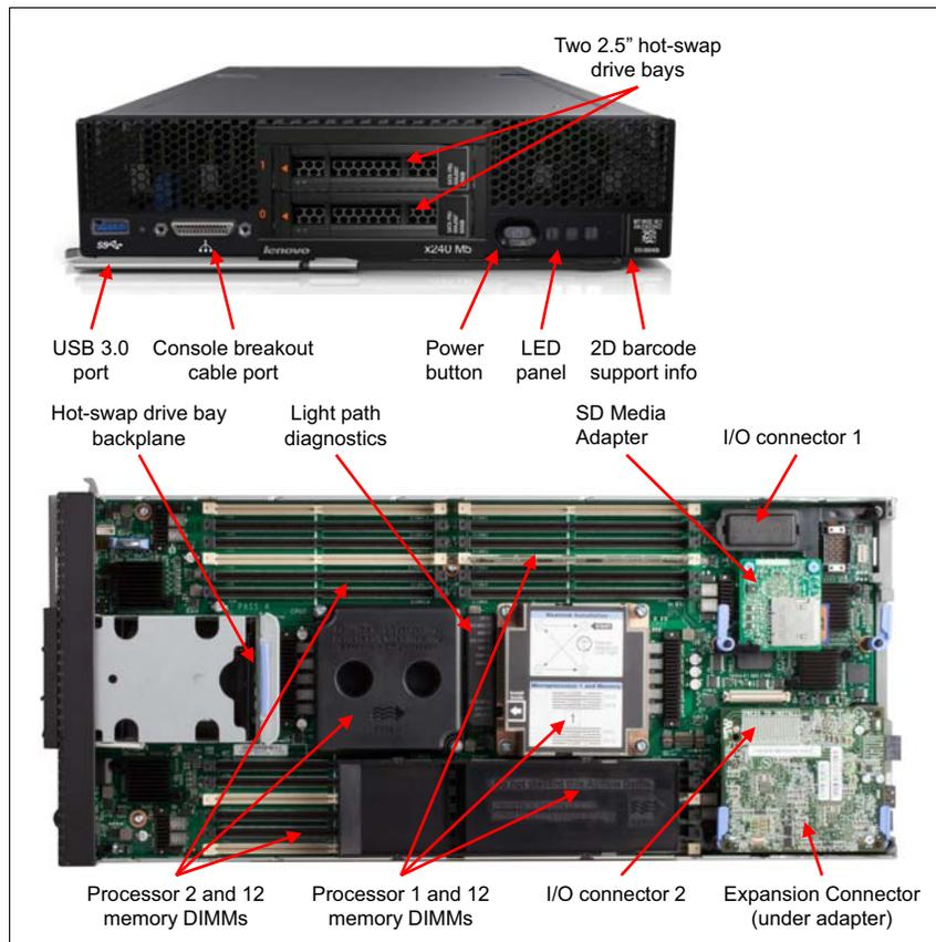
Figure 3-2 Flex System x240 M5
