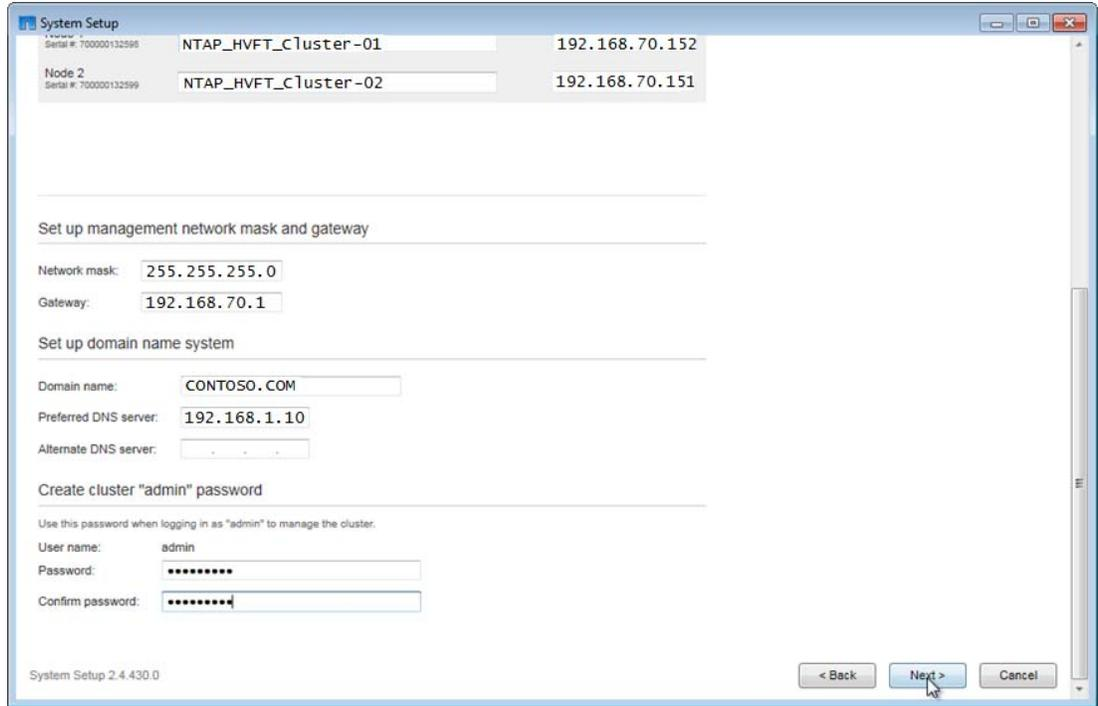
Figure 5-7 Assigning names and network addresses for storage
