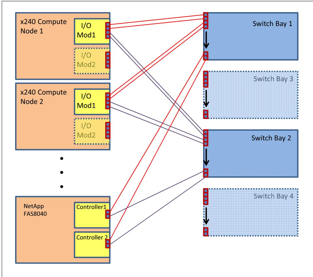
Figure 4-3 Converged storage and server connections
