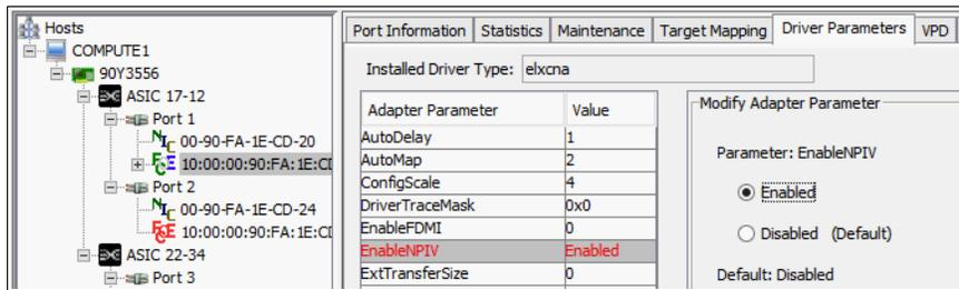
Figure 6-16 Enabling NPIV on FC ports
