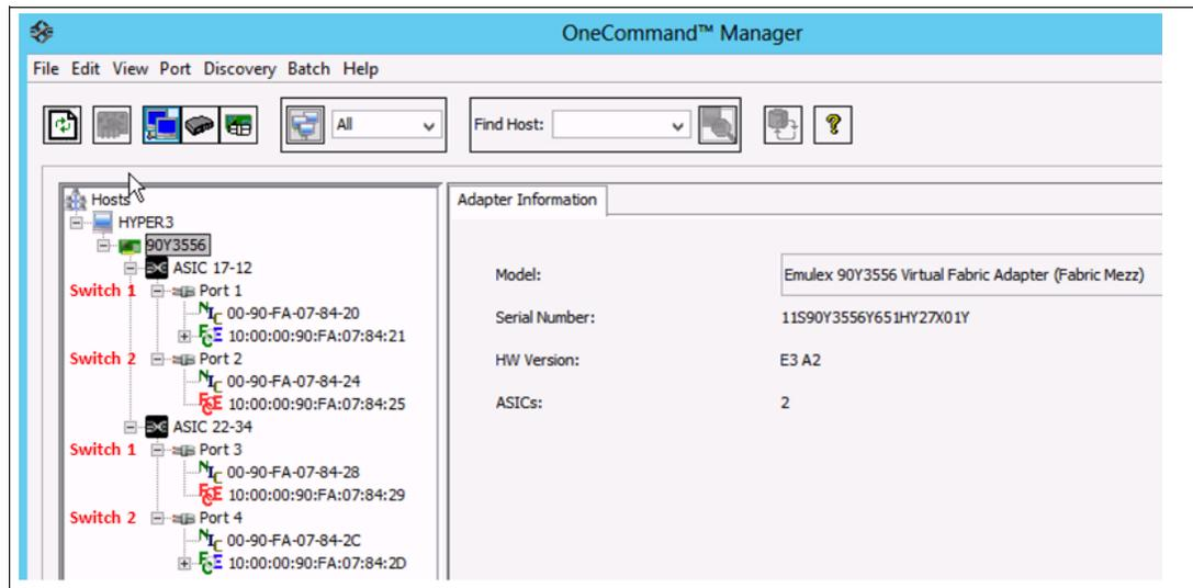
Figure 4-2 View of CN4054R network and storage connections
