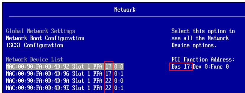
Figure 6-5 Identifying CNA devices to be configured
