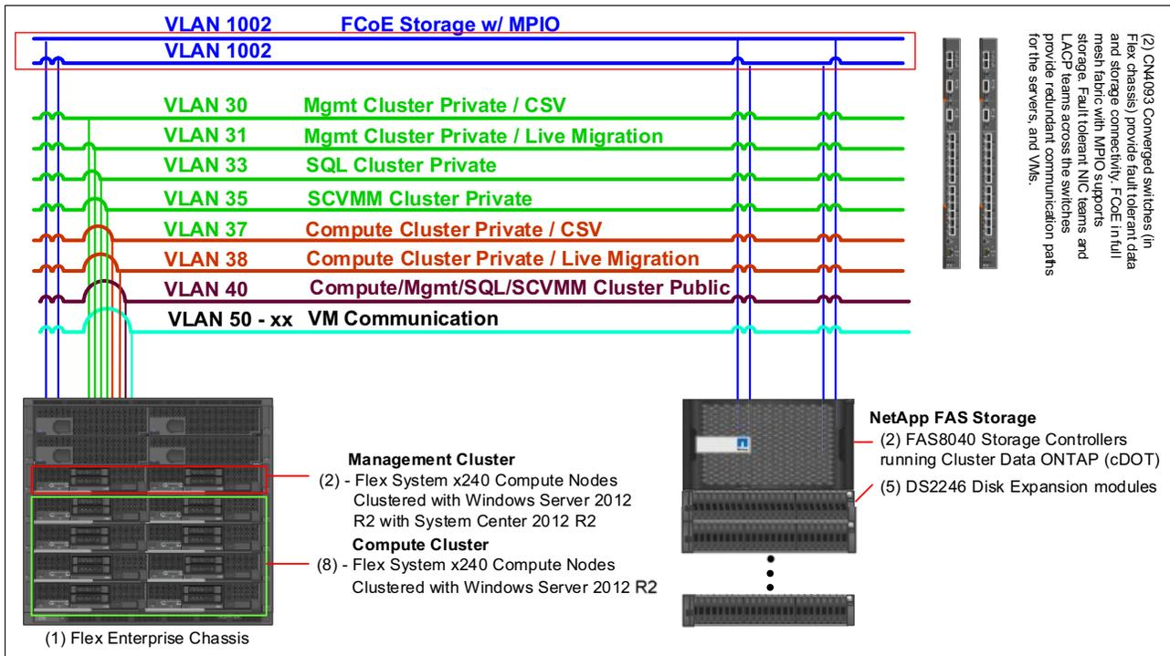
Figure 4-5 Flex System Solution for Microsoft Hyper-V architecture
