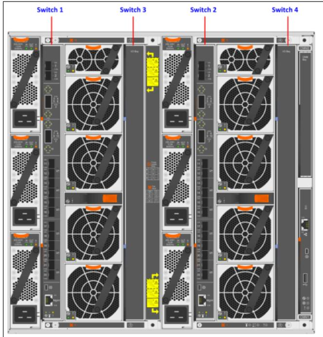
Figure 4-1 Flex System chassis switch position
