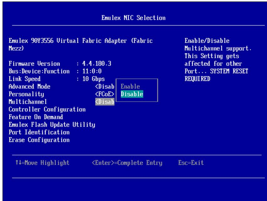
Figure 6-4 Disabling Multichannel Mode in CN4054R in UEFI
