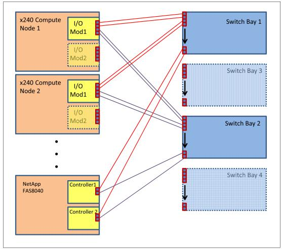
Figure 4-3 Converged storage and server connections
