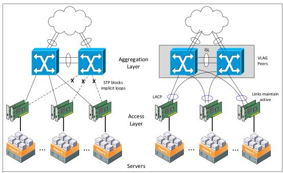
Figure 4-4 Typical data center switching layers with STP versus LACP
