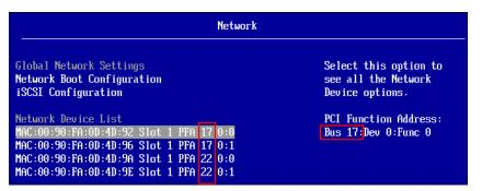
Figure 6-5 Identifying CNA devices to be configured
