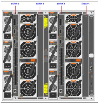
Figure 4-1 Flex System chassis switch position
