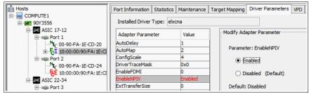
Figure 6-16 Enabling NPIV on FC ports
