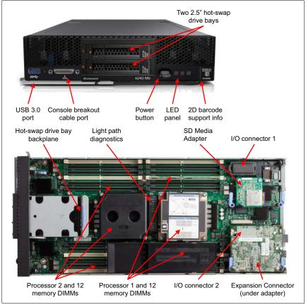
Figure 3-2 Flex System x240 M5
