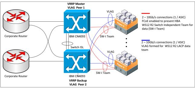
Figure 4-6 Active-Standby uplink configuration that uses LACP
