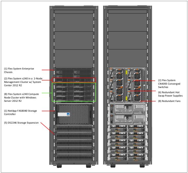
Figure 1-1 Lenovo Hyper-V Fast Track reference configuration
