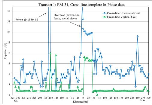
Figure 6.6: Cross-line to the SE-NW transect line. Figure 6.6a: conductivity data express the same anomalies with the in-line data plot. The metallic interferences around the SE 15m to NW 5m and with fence near -155m are better expressed on the cross-line conductivities. Figure 6.6b: Cross-line In-phase data becomes more sensitive when the EM-31 meter is in horizontal position. All the anomalies and metallic interferences are the same with the in-line plot.
