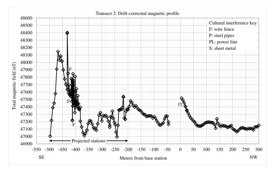
Figure 5.5. Magnetic profile of Transect 2, corrected for drift using repeat measurements at the 0 m and the +100 m (NW) stations. Readings were taken at every 5 m mark with an Overhauser GSM-19 Magnetometer. The locations of large metal objects were noted in the field and are marked on the profile as cultural interference. The noise between -380 m and -440 m is due to overlapping station locations that were measured off of the transect and then projected back onto the transect.
