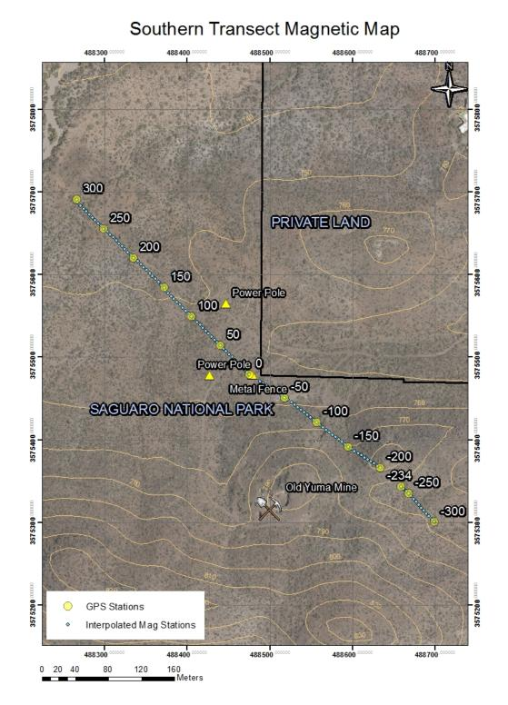
Figure 2.4. Transect 1 magnetic station map showing interpolated magnetic stations, contours, public/private land boundary, cultural interference, and GPS stations measured every 50m.
