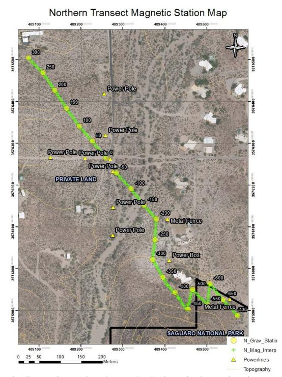
Figure 2.5. Transect 2 magnetic station map showing interpolated magnetic stations, contours, public/private land boundary, cultural interference, and GPS stations measured every 50m.
