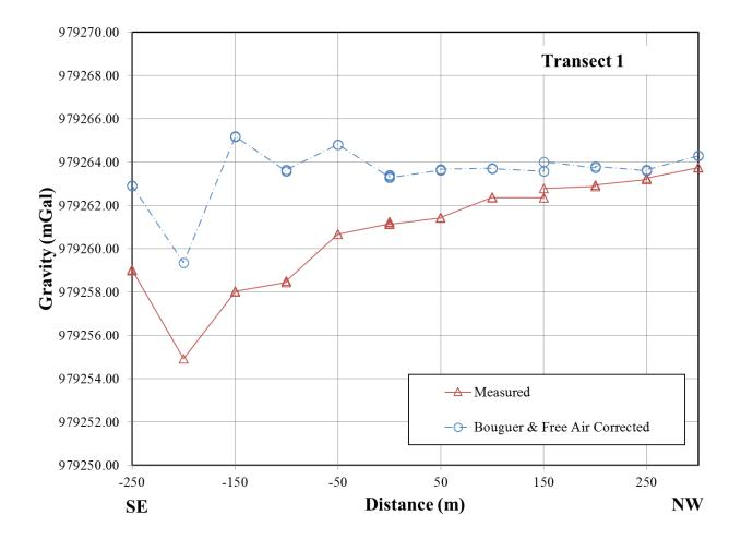
Figure 4.1 Measured gravity before and after Bouguer and free-air correction for transect 1.
