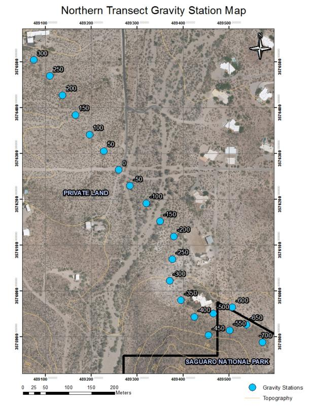
Figure 2.3. Gravity stations and topographic contours on satellite imagery. Note deviation due to house; measurements taken with permission on private land.
