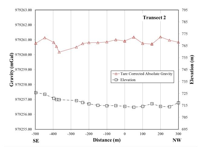
Figure 4.4 Gravity and elevation over distance for transect 2.
