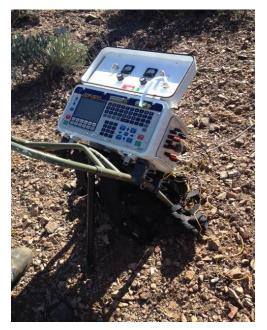
Figure 3.1. Zonge GDP-3224 multi-function receiver attached to the TEM/3 receiving antenna (not shown).
