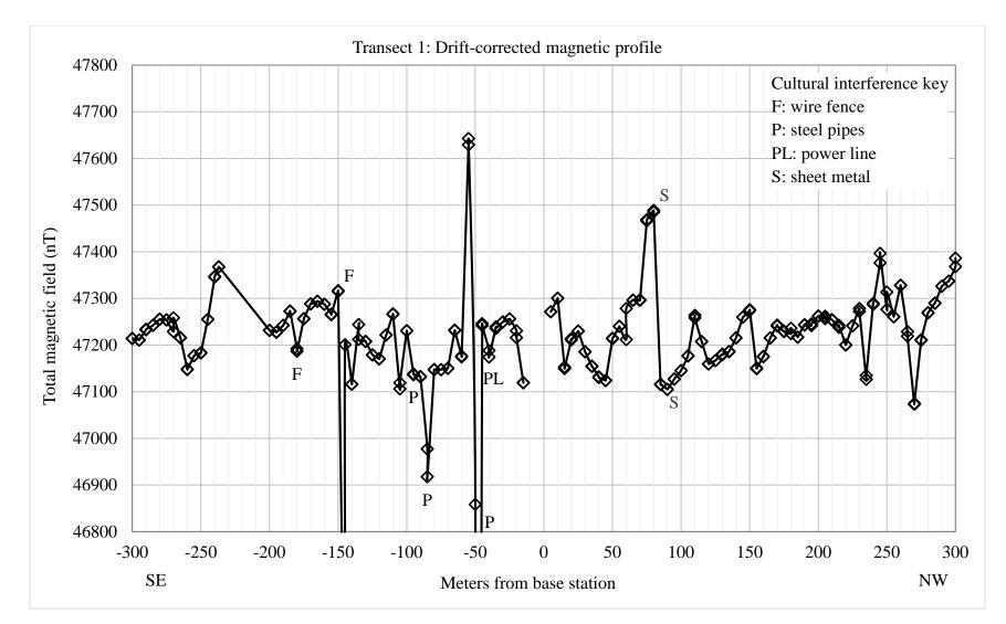
Figure 5.4. Magnetic profile of Transect 1, corrected for drift using repeat measurements at the +50 m (NW) station. Readings were taken at every 5 m mark with an Overhauser GSM-19 Magnetometer. The locations of large metal objects were noted in the field and are marked on the profile as cultural interference.
