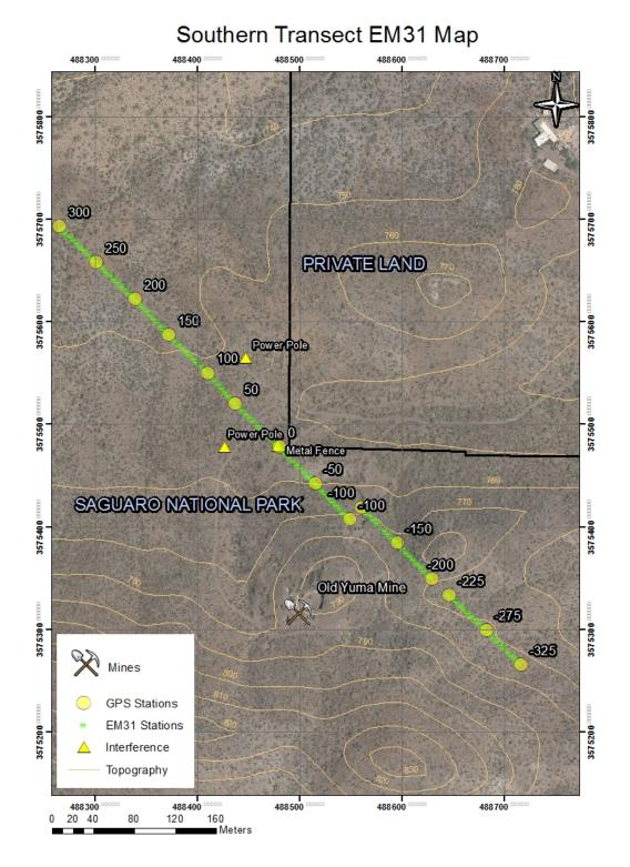
Figure 2.8 EM31 station interpolation shown. Sources of interference marked again with yellow triangles, interpolated stations shown with green asterisks. Additional information includes mine location, topographic contours, and GPS station measurements as well as land boundaries.
