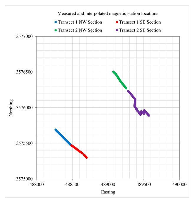
Figure 5.1. Location map for magnetic field measurements. Survey coordinates were recorded at every 50 m mark along each transect and were later interpolated to every 5 m.
