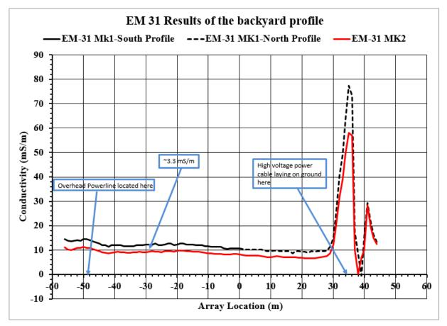
Figure 6.1: EM 31: MK-1 & MK-2 data plot from a test-site, conducted to check the equipment's functionality and to compare the output between the two models of EM-31. Only the in-line, horizontal coil test was performed at the test site. Neither the cross-line, nor the vertical surveys were performed.
