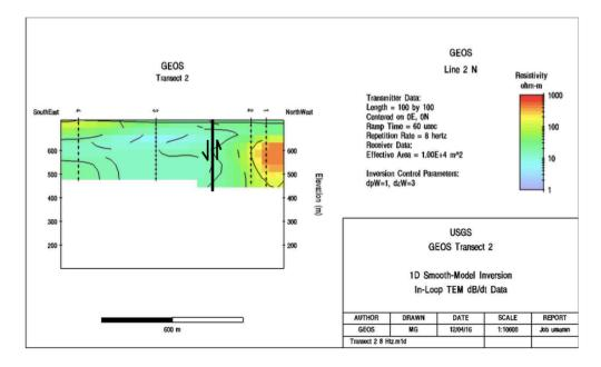
**Figure 8.1.** The 8-Hz. TEM modeled cross-section from Transect 2, with an approximate location for the normal fault detected between stations 2 and 3. This fault may be a subsurface continuation of the fault interpreted near the mine by Lippman (1993).
