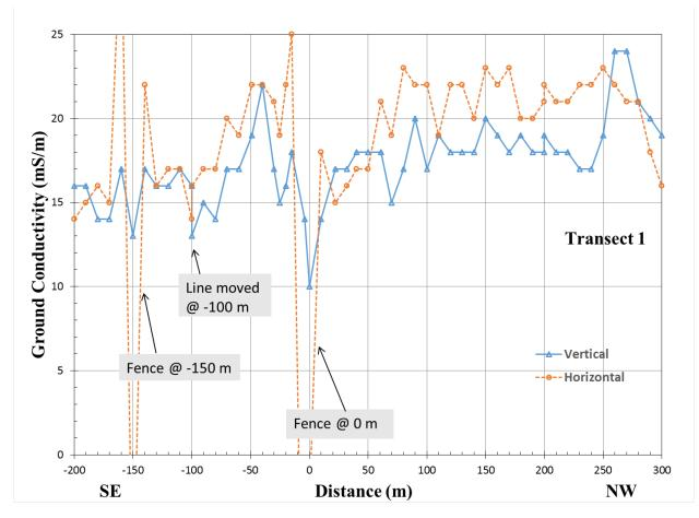
Figure 7.2. Zoomed-in EM34 measured ground conductivity (mS/m) over distance for transect 1.
