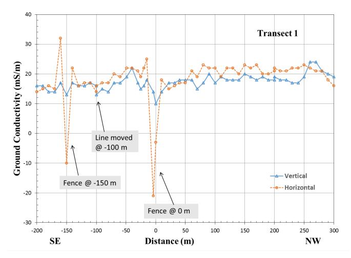
Figure 7.1. EM34 measured ground conductivity (mS/m) over distance for transect 1.
