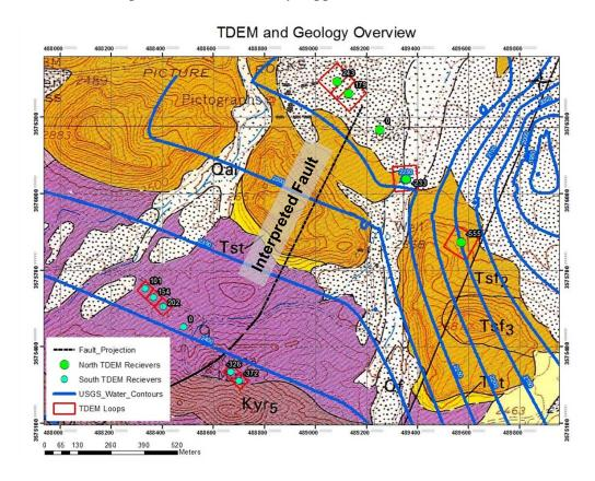
Figure 8.2. Projected fault line location based on TEM data with water contours and local geology (Lipman, 1993).
