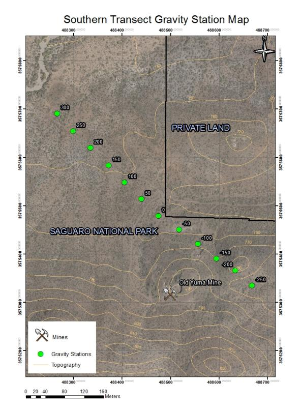
Figure 2.2. Gravity station locations with satellite imagery and topographic contours. Also displayed are private and public land boundaries. In this particular location measurements were not allowed to be taken on the adjacent private land.
