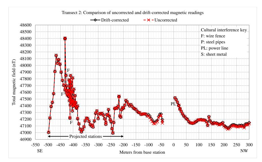
Figure 5.3. Magnetic profile for Transect 2, demonstrating the magnitude of the applied drift correction. Readings were taken at every 5 m mark with an Overhauser GSM-19 Magnetometer. The locations of large metal objects were noted in the field and are marked on the profile as cultural interference. The noise between -380 m and -440 m is due to overlapping station locations that were measured off of the transect and then projected back onto the transect.
