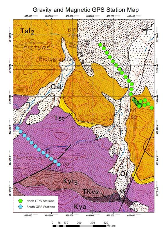
Figure 2.1: Geology map of the area (Lipman, 1993). Data points containing every measured GPS point for the gravity and magnetic stations are displayed on the map.
