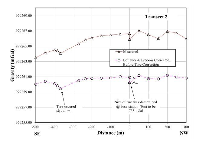
Figure 4.3 Measured gravity before and after Bouguer and free air correction for transect 2, with indication for the occurrence and size of tare (not corrected in the figure).
