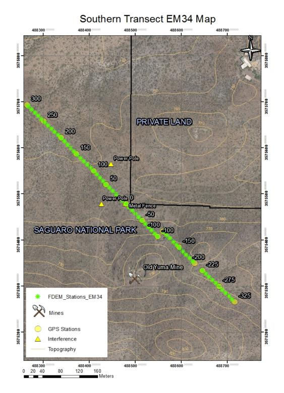
Figure 2.9 EM34 station interpolation shown. Sources of interference marked again with yellow triangles, interpolated stations shown with green asterisks. Additional information includes mine location, topographic contours, and GPS station measurements as well as land boundaries.
