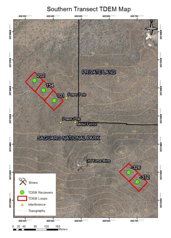
Figure 2.6. TEM receiver stations shown with loop corners on satellite imagery with topographic contours. Cultural interference areas indicated with yellow triangles.
