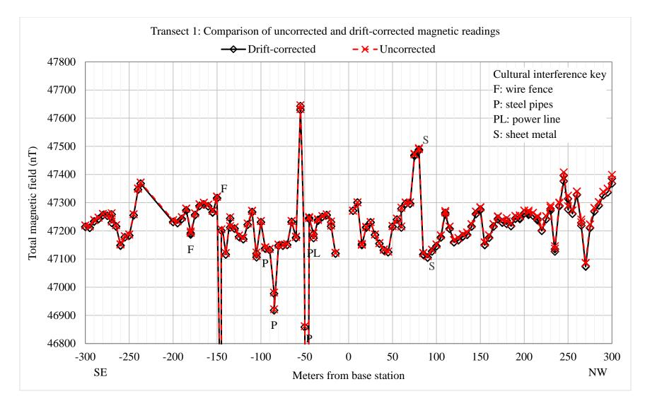
Figure 5.2. Magnetic profile for Transect 1, demonstrating the magnitude of the applied drift correction. Readings were taken at every 5 m mark with an Overhauser GSM-19 Magnetometer. The locations of large metal objects were noted in the field and are marked on the profile as cultural interference.
