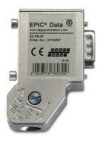
EPIC® Data PROFIBUS connectors are screw terminal, 9 pin D-Sub connectors with an integrated adjustable termination resistor. The cable entry is 35° angled. Connectors are available with additional programming/diagnostic interface.
