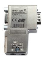
EPIC® Data PROFIBUS connectors are spring-type, 9 pin D-Sub connectors with an integrated adjustable termination resistor. The cable entry is 90° angled. Connectors are available with additional programming/diagnostic interface.
