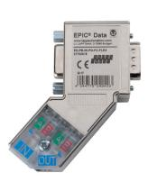
EPIC® Data PROFIBUS connectors are fast connect, 9 pin D-Sub connectors with an integrated adjustable termination resistor. The cable entry is 35° angled. Connectors are available with additional programming/diagnostic interface.
