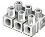
G T1281/3 Three way terminal block. Each way will accept one 2.5sq mm cable or two 1.5sq mm cables together.
