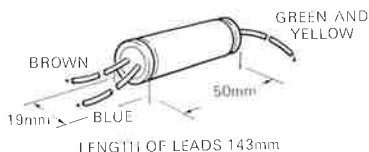
G C2051 A radio interference suppression filter network comprising two 0.005µF and one 0.1µF delta connected for additional suppression where the GC2139 fails to suppress the interference.
