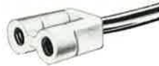
G M6064/12/Loop Starter Socket White PVC moulding enclosing starter switch contacts crimped to 12in loop of 0.5sq mm white PVC cable which can be cut at a point to suit wiring layout. Current item for 2ft fittings and for earlier Popular Pack fittings in other sizes.
