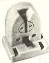
K7221 Fixed Bi-Pin Lampholder. K7221E Fixed Bi-Pin Lampholder with earth contact. Screw fixing. Material: Philite White. Electrical Connections: K7221 Push-wire terminals. K7221E Push-wire terminals.
