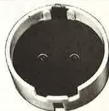
K7265E Bi-Pin Push-on fully shrouded lampholder with earth contact. Material: Urea. Electrical connections: Push-wire terminals. Earth contact: Screw terminals.
