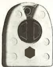
K7202 Fixed Bi-Pin Lampholder. Screw Fixing to Back Plate. Material: Philite White. Electrical connections: Push-wire terminals.
