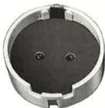
K7265E Bi-Pin Push-on fully shrouded lamp holder with earth contact. Material: Urea. Electrical connections: Push-wire terminals. Earth contact: Screw terminals.
