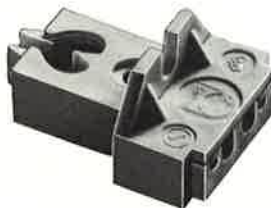
K7229/1 Fixed Bi-Pin Lampholder for 16mm miniature lamps. Screw fixing. Material: White Polypropylene. Electrical connections: Push-wire terminals.
