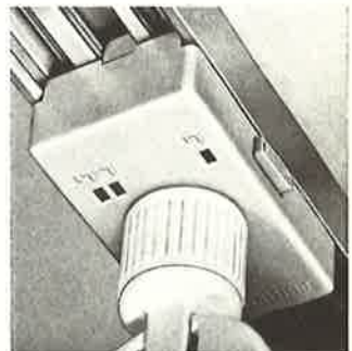
The body simply plugs into the track, and is released by depressing two side catches. The adaptor is unobtrusive and simple, with no switches or fuse.
