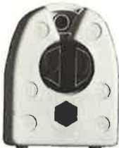
K7202 Fixed Bi-Pin Lampholder. Screw Fixing to Back Plate. Material: Philite White. Electrical connections: Push-wire terminals.
