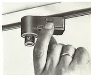
Loose adaptor RCS 655/12 (including cord grip) is simply fitted by pressing adaptor at right angles onto track and turning it through 90° to left or right (depending on circuit required).
