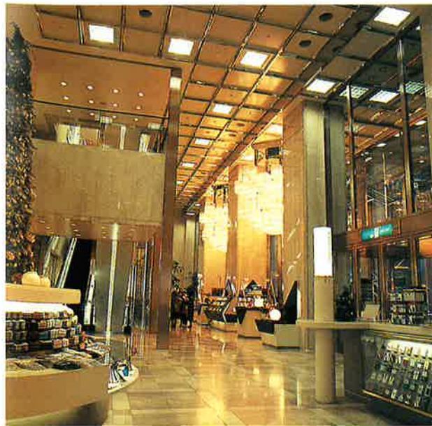
Mixed lighting using EYE Specialux and EYE Multi-Metal Lamps This is widely used in stores and commercial displays as it features superior color rendering properties.
