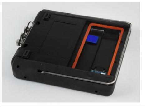
4. To remove the memory card, push the memory card into the memory card slot until it clicks and releases.
