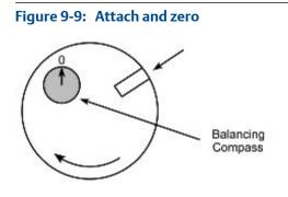
3. Turn the rotor until the indicator reads the desired angular position from the applicable scale. This position is now aligned with the stationary reference.
