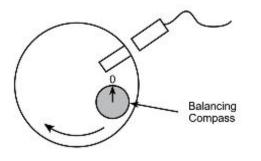
4. Turn the rotor until the reference mark is at TDC.
