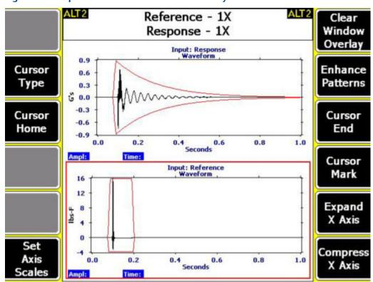
Figure 6-4: Impact waveform with window overlays
