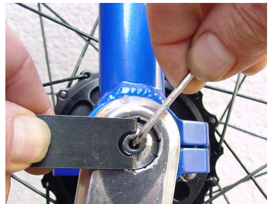
Picture 7: Hold the gear shift button with the black wrench and tighten it well with an 2.5 Allen wrench
