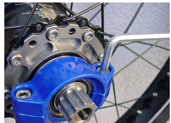
Picture 4: Tighten the screws evenly with 5-6 Nm!
