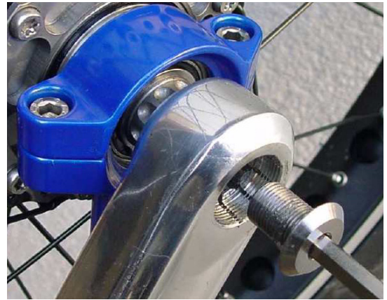
Picture 5: Mount crankarm and adjust axle bolt
