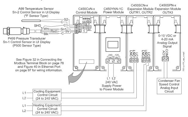
Figure 10: Example System 450 Control with Communications Showing a Room Heating and Cooling Application with Condenser Fan Speed Control
