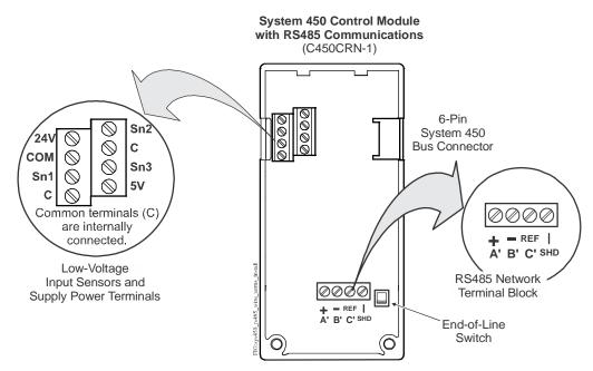
Figure 16: C450CRN-1 Control Module with Modbus Communications Showing Wiring Terminals
