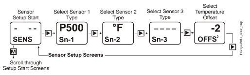
Figure 23: Sensor Setup Start, Select Sensor Type, and Select Temperature Offset Screens
