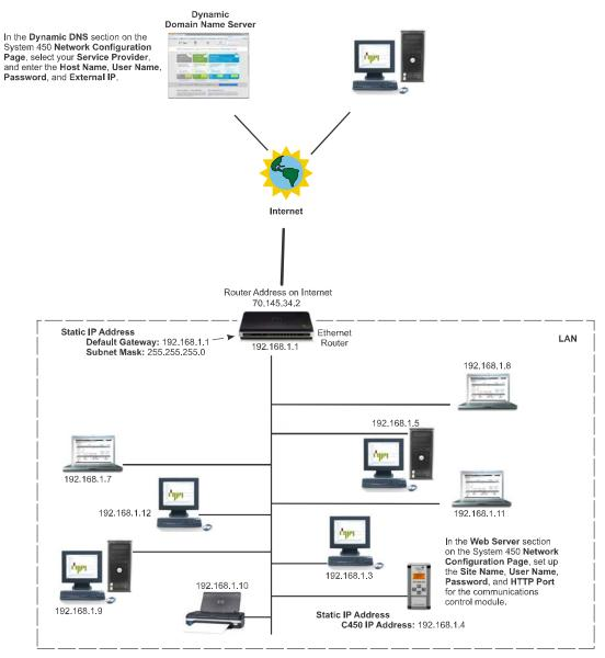
Figure 42: Example Network Diagram with System 450 on a Local Network
