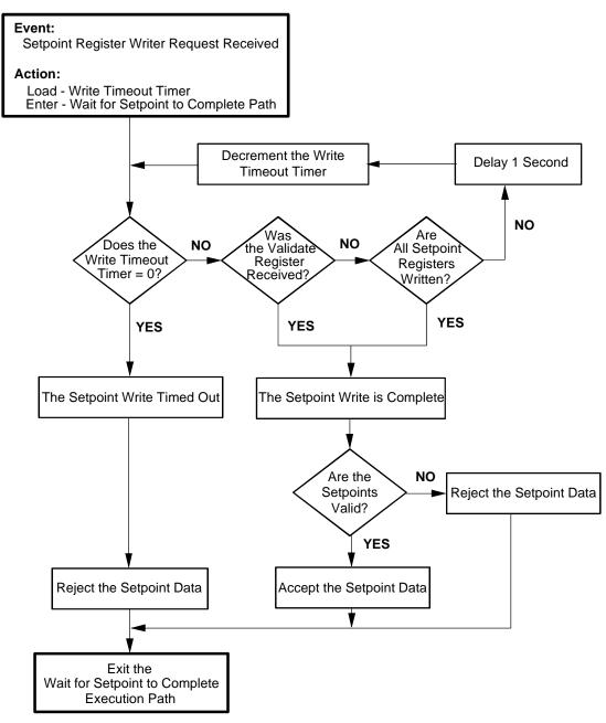
Figure 39: Setpoint Wiring Flowchart
