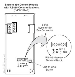
Figure 32: C450CRN-x Control Module with Modbus Communications Showing Wiring Terminals, Input Terminals, and Network End of Line Switch
