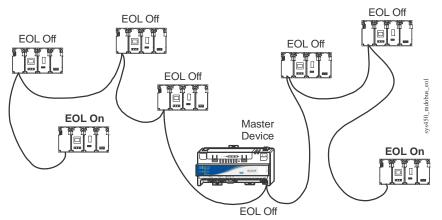
Figure 34: EOL Switch Settings on an Example Modbus Network Trunk
