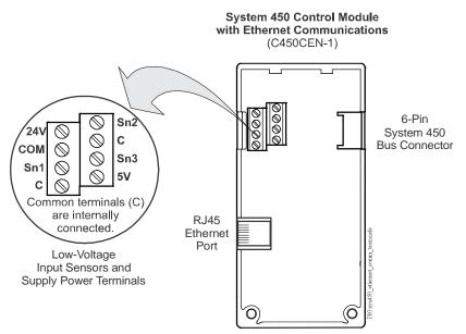
Figure 17: C450CEN-1 Control Module with Ethernet Communications Showing Wiring Terminals
