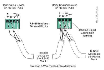
Figure 33: Modbus Terminal Block Wiring Detail
