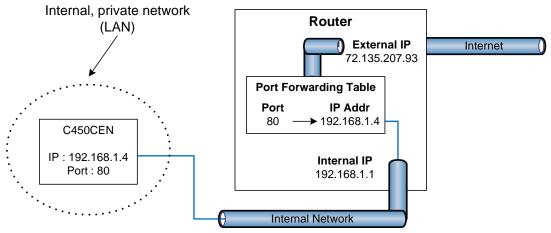
Figure 43: Port Forwarding Configuration Example
