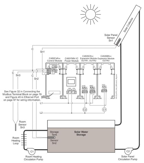
Figure 14: Example System 450 Control with Communications Showing a Solar Water Space Heating Application that Uses the Differential Control Feature
