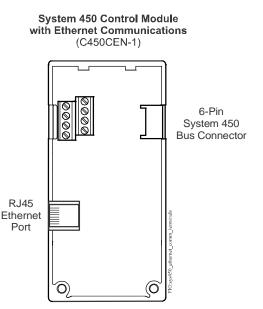
Figure 40: C450CEN-1 Control Module with Ethernet Communications Showing Input Wiring Terminals and Ethernet Port
