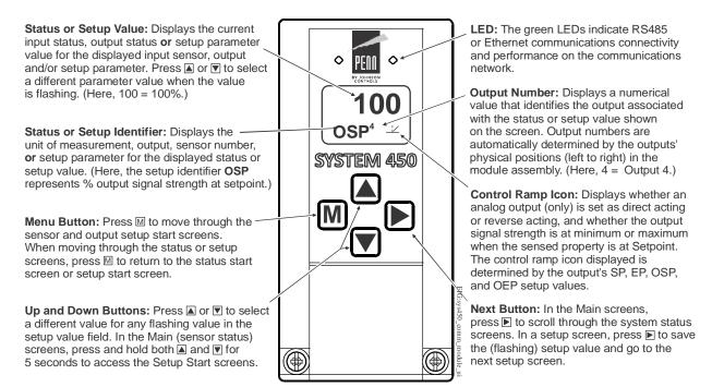
Figure 2: System 450 Communications Control Module Showing LCD and Four-Button Touchpad User Interface
