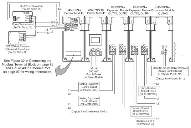
Figure 12: Example System 450 Control with Communications Showing a Clean Room Application that Controls Temperature, Pressure, and Humidity Simultaneously
