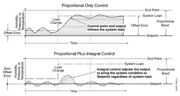
Figure 7: Proportional Only Control Versus Proportional Plus Integral Control
