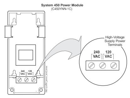
Figure 20: System 450 C450YNN-1C Power Module Showing High-Voltage Supply Power Terminals
