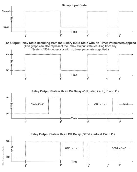
Figure 5: Behavior of a Relay Output Referencing a Binary Input or Other System 450 Compatible Sensor and the Resulting Output States with the On Delay and Off Delay Parameters Applied The bottom two graphs in Figure 6 show an example of the relay output behavior when the Minimum On or Off Time parameter is applied to the relay output (regardless of whether the relay output references a binary input or another compatible sensor).
