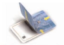
Illustration showing the antenna inside a smart card and that the card can be used for photo ID.
