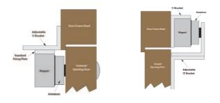
These are now the most commonly used access control lock due to their ease of installation and tolerance to door deterioration. These locks are by their design 'FAIL-SAFE' units. This means that they require the power from the access system to provide a holding force. When the power is removed the lock releases. Should there be a total power failure, cable damage etc, the lock fails in a released state. The locks in this section are face to face style.
