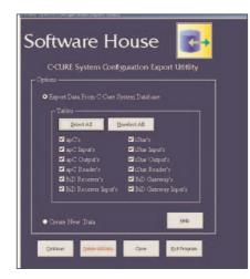
The C•CURE Configuration Import/Export Utility is a tool that allows customers to design and load security objects into the C•CURE 800/8000 system.
