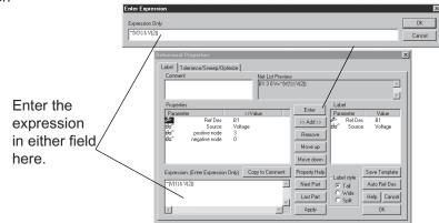
NAND Gate .TRAN 1U 2.5M BNAND 3 0 V=~(V(1)&V(2)) V1 1 0 PULSE 0 5 0 1U 1U 100U 200U V2 2 0 PULSE 0 5 0 1U 1U 200U 400U .END  Construct and simulate the NAND circuit. Notice how the voltage sources and the B element are not wired together. When the simulation is complete, examine the output.
