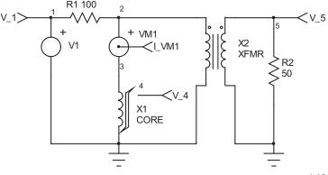
Saturable Core, Advanced Macro Modeling .SUBCKT CORE#0 1 2 3 RX 3 2 1E12 CB 3 2 1E-7 IC=-250 F1 1 2 VM1 1 G223121 E142321 VM145 RB 5 2 100K RS 5 6 200 VP 7 2 250 D1 6 7 DCLAMP VN 2 8 250 D2 8 6 DCLAMP .MODEL DCLAMP D(CJO=191P VJ=25) .ENDS
