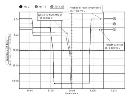
See the Alter dialog for more information on sweeping the circuit temperature. temperature set in the .OPTIONS statement. With this feature, it is easy to simulate a device at one temperature, and the rest of the circuit at another temperature.
