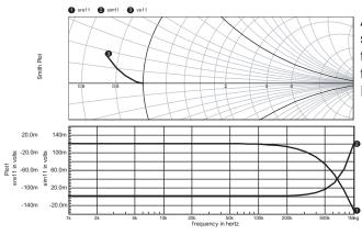
A Smith Chart and a plot of the sre11 and sim11 waveforms are the result of selecting vs11 in the Smith Chart submenu of IntuScope's calculator.
