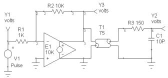
resistors, R1 and R2, create a simple inverting amplifier configuration with a gain of 10. This inverting amplifier essentially buffers the input voltage source to the transmission line.
