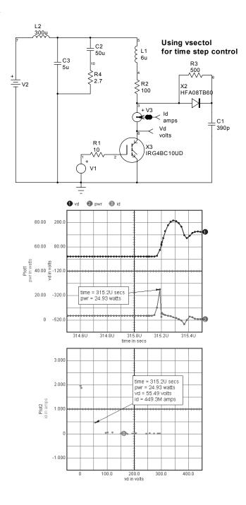
Results using VSECTOL to control the time step produces higher accuracy during the turn-off transition and uses less computational resources when there is no switching activity.
