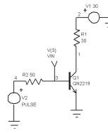
Open up the drawing at :\spice8\ Circuits\ Examples\ Temperature.DWG Use the Properties dialog to enter the values for TC1 and TC2 for RMOD. The dialog will generate the RMOD .Model statement. Simulating at Different Temperatures \*#SAVE ALL ALLCUR ALLPOW .MODEL RMOD R(TC1=.01 TC2=1E-6) .PRINT TRAN V(3) R1 1 2 30 RMOD ; enter Rmod in the .Model Value field V1 2 0 30 R2 3 4 50 RMOD V2 4 0 PULSE 0 5 0 10N 10N 500N 1U Q1 1 3 0 QN2219 .END
