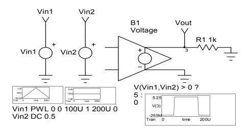
The B element can be used directly in a schematic, however, it has no nodal input connections making schematic capture arkward. This is due to the fact that the input to a B element is an arbitrary expression and can be made of node voltages, device currents, and other quantities.
