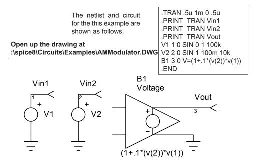
We could have generated a current output with the B source by replacing "v=" with "i=". For example, B130I=(1+.1\*(v(2))\*v(1)).
