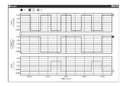
The .OPTIONS parameters, LTHRESH, LONE and LZERO control the turn-on/turn-off voltage threshold, the high level output and low level output, respectively.
