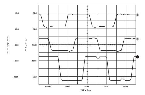
is done by setting R to a nonzero value. Unfortunately, it is not as easy as plugging in a value. If R is included, the characteristic impedance (Zo), and phase velocity (Vp) will change. This will change the values of L and C. For this example, however, we will simply add a unit resistance of  $4\Omega$ /m and simulate the circuit for a 50m line.
