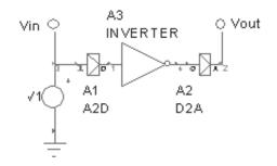
• Double-click on the voltage source then double-click on "None" in the Tran Generators option to enter the following values.
