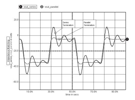
• To improve the matching, replace the  $150\Omega$  resistor and 10pf capacitor with the parallel termination shown to the left. Simulate the circuit again. The new statements are shown below for reference.
