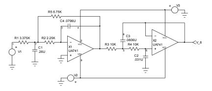
The UA741 is located in the Part Browser dialog under the Op-amps Part Type, Intusoft Sub Type listing.
