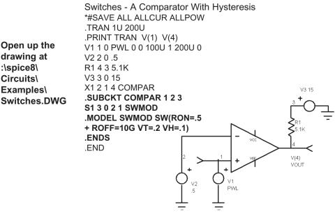
Current controlled switches are also available in IsSpice4. As you can see, a different approach was used for this comparator. The switch model in IsSpice4 is used because it contains parameters to model hysteresis. Since the hysteresis is built into the switch model, the construction of a comparator with hysteresis becomes quite easy.
