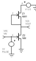
The .PRINT, statement is entered in the User Statement field in the IsSpice4 Simulation Setup dialog. must be made, one for "MN" and one for "MN1." If the model was the same for both devices, then only one .MODEL line would be needed. You can enter the model parameters for each MESFET through the MESFET's Part Properties dialog. The parameter values can be seen from the netlist on the previous page.
