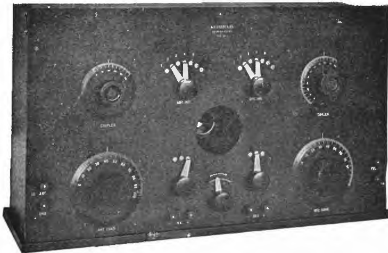
FIG. 207a. Grebo type C R 7 long wave receiving set. Range 500 to 20,000 meters.
