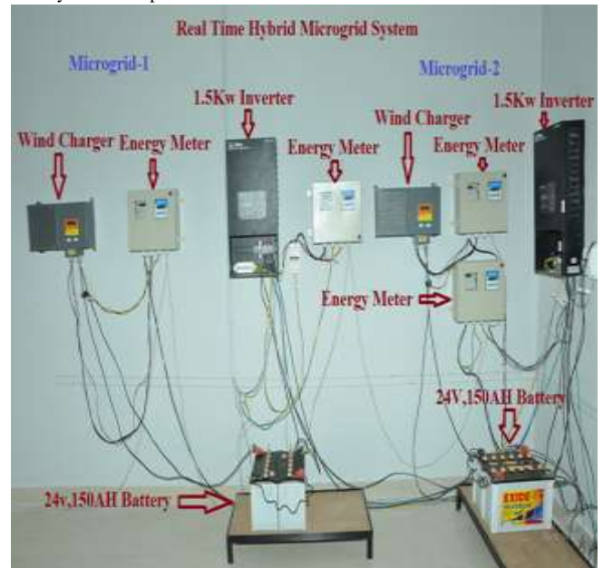
Fig.3. Proposed micro-grid control system installed in power system research laboratory of EEE department.
