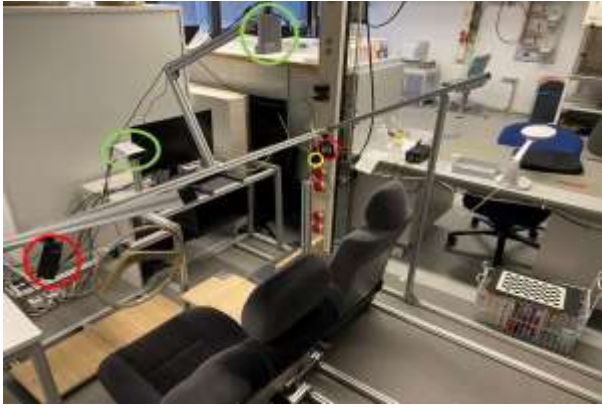
Fig. 2. Vehicle mock-up - The sensors installed in the mock-up includes two Azure Kinect (green circles), two radars (red circles) and one fish-eye lens camera (yellow circle)
