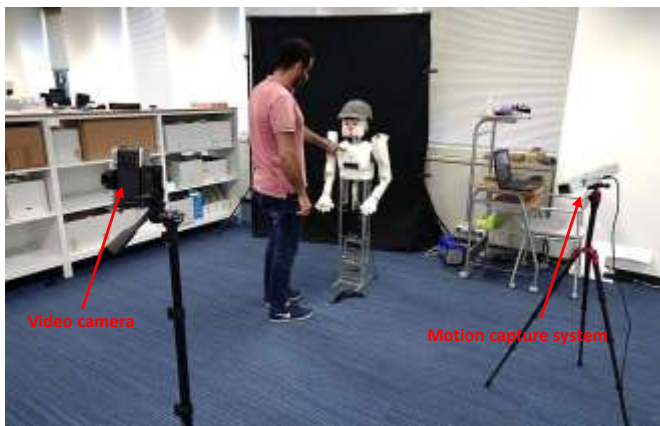
Fig. 8. Experimental settings of the poking experiment.
