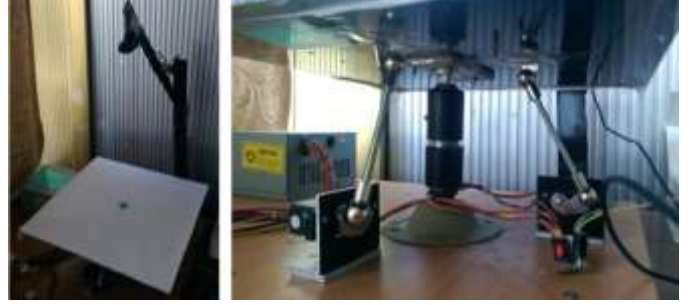
Fig. 7. The stand for balancing the ball on the platform.
