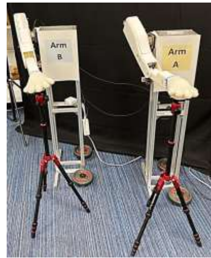
Fig. 12. Experimental setups of the high five experiment.
