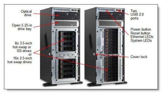
Figure 2. Front view of the IBM System x3300 M4 server
