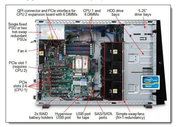
Figure 4. Inside view of the IBM System x3300 M4 server
