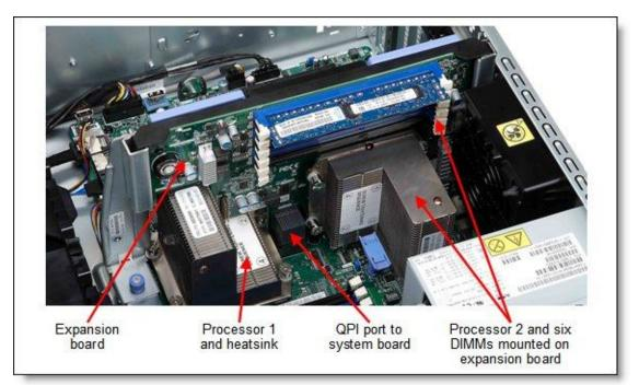
Figure 5. Processor 2 installed on the expansion board
