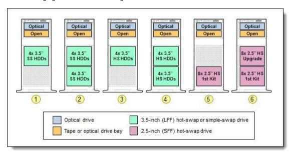
Figure 6. Internal drive configurations
