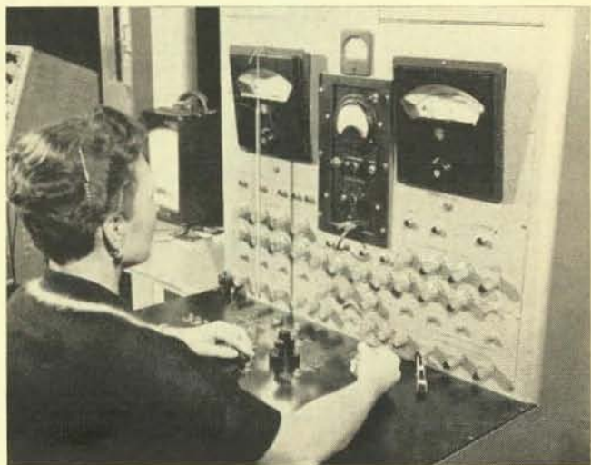
Here is one of the pieces of test equipment used to check each transistor prior to shipment.
