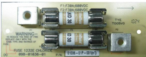
Fuse board PCB
