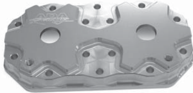
KA750 KAWASAKI 800SXR/750 NON-GIRDLE BILLET HEAD SHELL
