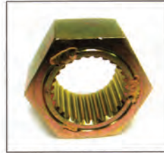
Drive Shaft Adaptor Part No. 950-120 O.E. No. 529-035-985 Fits: RXP 4 Tec
