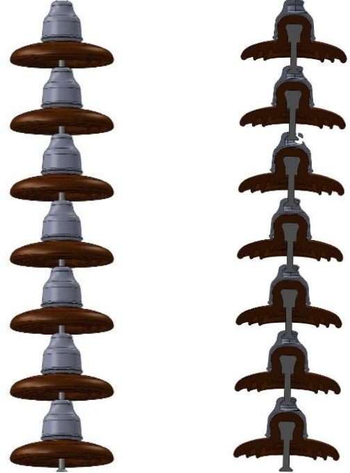
Fig.4. The suspension insulator type 52-3 and the cutting plane of the suspension insulator model
