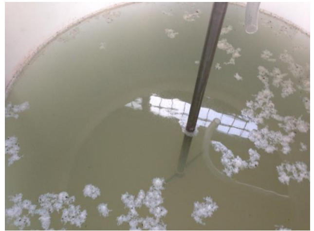
Fig 5. Supernatant after settling for 1 hour
