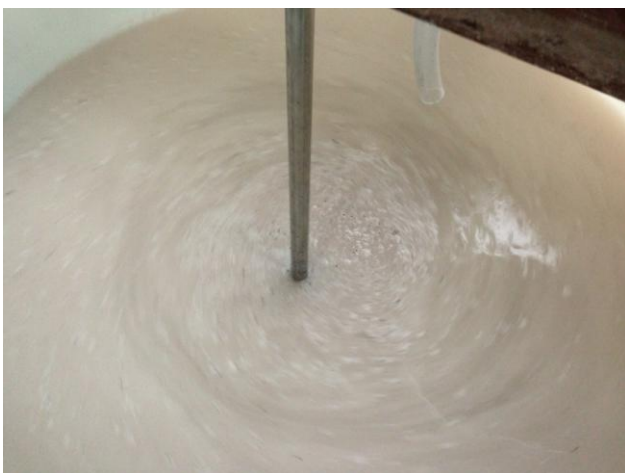
Fig. 4. Rapid mixing and slow mixing with stainless steel paddle and control speed with electric motor.
