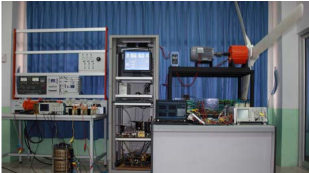
Fig.6. Power Quality Controller and Compensate of Wind Turbine Generation
