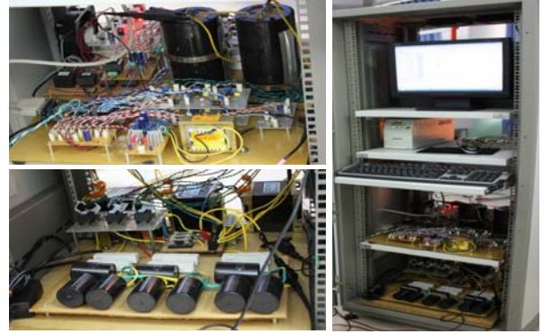
Fig.5. Hardware Prototype of the Proposed STATCOM
