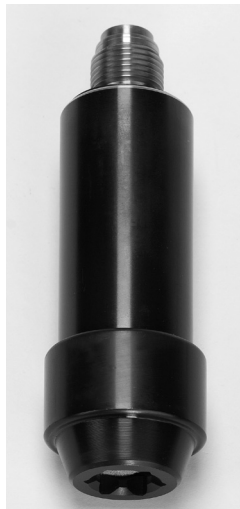
SIoux STANDARD 3/8" + .010 (.385") upper end size. 1 1/16" x 16 thread. Part No. K-1702
