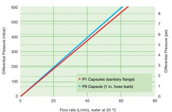
For liquids other than water, multiply differential pressure by fluid viscosity (cP).
