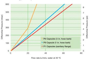
For liquids other than water, multiply differential pressure by fluid viscosity (cP).
