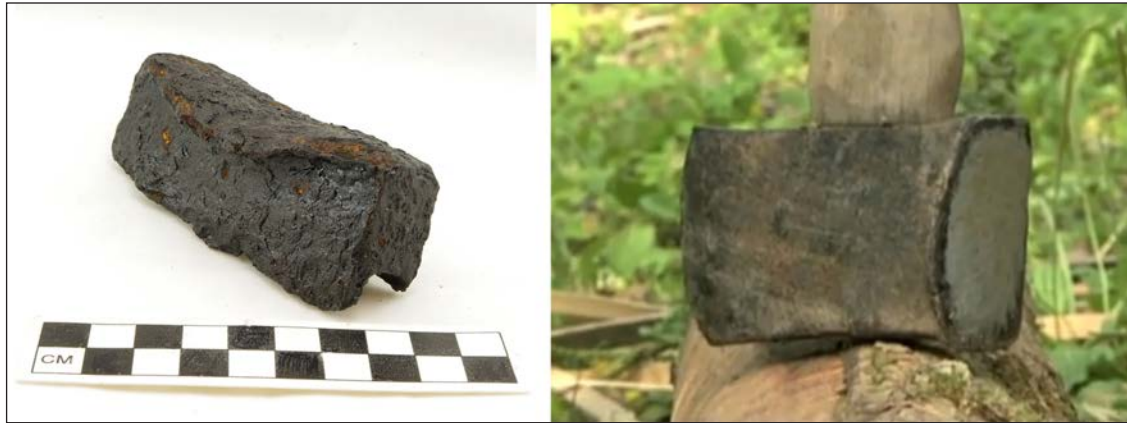
Figure 8-22. Axe head showing warping from use.
