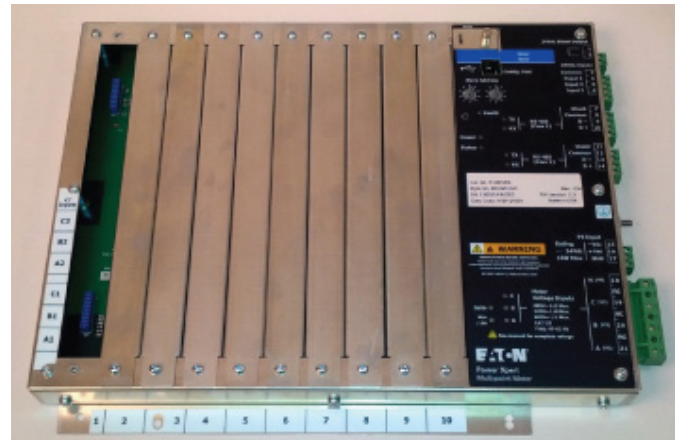
Figure 36. Cover Plate Removed from Slot 1.
