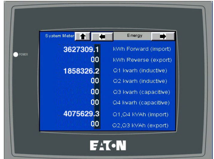
Figure 87. Meter Energy Information Displayed When a Specific Sub-Meter Is Selected.
