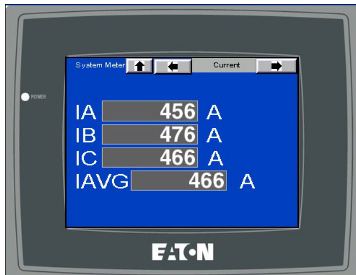
Figure 75. The System Meter Current Screen – The First System Meter Function Screen that Appears.
