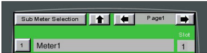
Figure 85. The Location of the Page and Sub Meter Selection Buttons on the System Sub Meter Screen.
