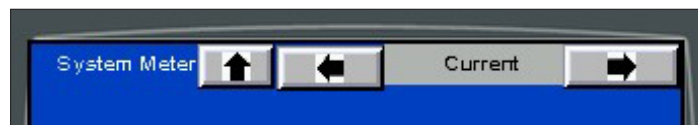
Figure 76. Back, Left, and Right Arrow Buttons Used to Navigate Through the Screens.
