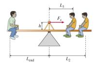
$WL_{end} - hF_{x} - w(L_{2} + L_{3}) = 0$  $F_{x} = (WL_{end} - w(L_{2} + L_{3})) / h$
