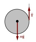
115. **Picture the Problem**: You pull straight downward on a rope that passes over a disk-shaped pulley and then supports a weight on the other side. The force of your pull rotates the pulley and accelerates the mass upward.
