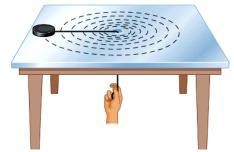
$mvr = mv_{\rm f}r_{\rm f}$  $v_{\rm f} = v \left( \frac{r}{r_{\rm c}} \right) = v \left( \frac{r}{\frac{1}{2}r} \right) = \boxed{2v}$
