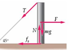
**Strategy:** Let *L* = the rod length and write Newton's Second Law for torque about the bottom of the rod in order to determine the wire tension *T*. Then write Newton's Second Law in the horizontal and vertical directions to determine the normal force *N* and the static friction force  $f_s$ . Then determine the maximum force *F* that can be applied to the rod without causing it to slip.
