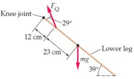
$$F_{\rm Q} = \frac{r_{\perp,\rm W}}{r_{\perp,\rm Q}} mg = \frac{27 \text{ cm}}{5.8 \text{ cm}} (3.4 \text{ kg}) (9.81 \text{ m/s}^2) = 155 \text{ N} = \boxed{0.16 \text{ kN}}$$
