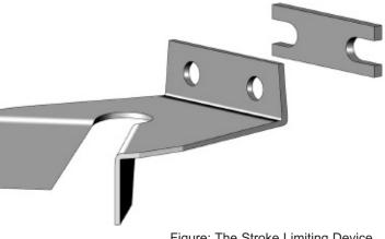
Figure: The Stroke Limiting Device complete with Stopper
