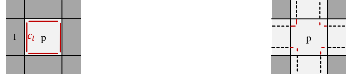
Fig. 1. Left: The 4 potential edge-parallel-CS-parts of a pixel p . c_l is set, if pixel l 's classification differs from p 's, for instance. Right: Link-CS-parts
