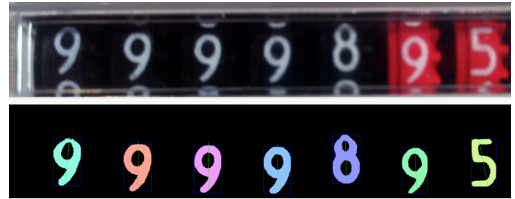
Figure 2. An example of the output of the algorithm after the "filter blob" step (top: original image, bottom: result).
