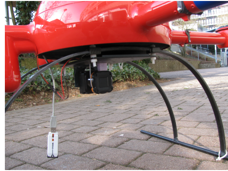
Figure 3: This figure shows how the laser scanner is mounted on the MAV (It is noted that the laser scanner is mounted such that the beam will be scanning downwards).
