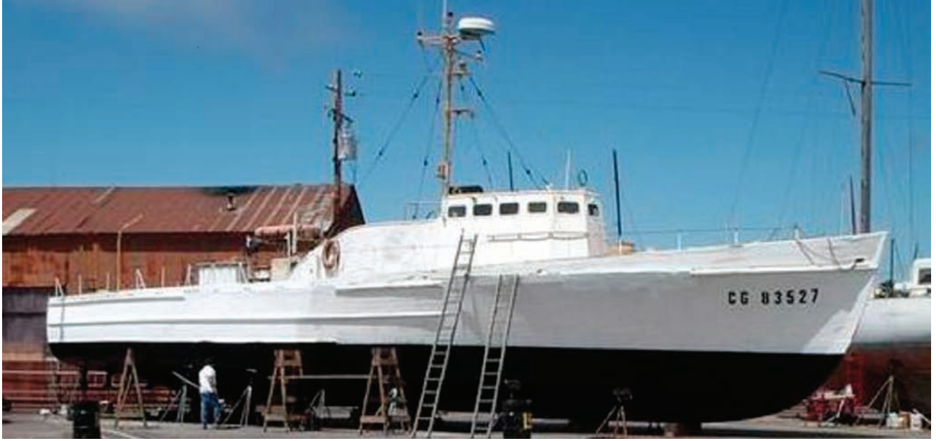
Prior to her 2004 return voyage to Puget Sound, the cutter CG-83527 was hauled out for inspection, hull repair, and painting at Bay Ship and Marine in Richmond, north of San Francisco. Preparations and sea trials were completed in June, and the trip up the coast began. Photo by Dan Withers.
