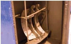
Individual shot blasting ensures 100% removal of external contaminants - necessary for reliable coating coverage.
