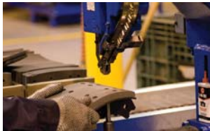
Rivet torque specifications are critically maintained to ensure reliable lining to shoe attachment.
