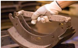
Shoe quality begins at core check-in. Out of spec shoes are scrapped.
