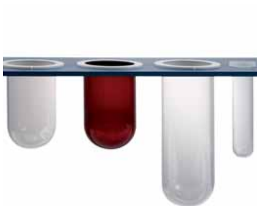
(Left to right) 1L TruAlign vessel, 1 L low actinic - red TruAlign vessel, 2 L TruAlign vessel and 200 mL TruAlign vessel
