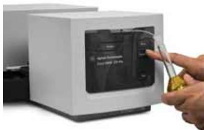
Sipper operation is easy with built-in measurement buttons.
