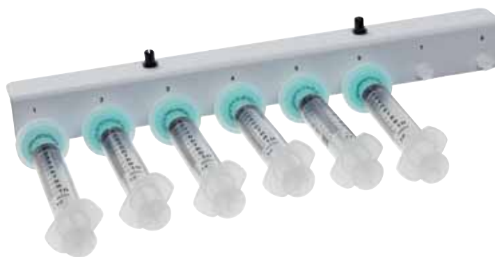
Manual sampling bracket for 708-DS or 709-DS Dissolution Apparatus
