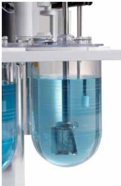
Custom basket used for preheating inside a DVH vessel
