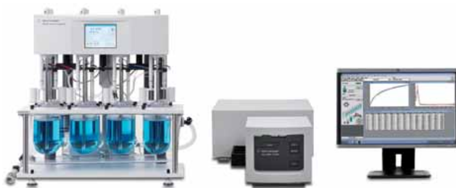
708-DS Dissolution Apparatus paired with the Cary 8454 UV-visible Spectrophotometer and UV-Chemstation Software
