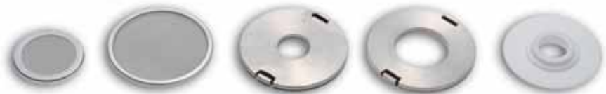
(Left to right) Paddle Over Disk assemblies, transdermal patch holders and suspension cup.
