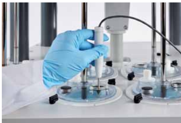
Manual temperature measurement using 708-DS temperature probe.
