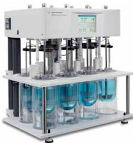
709-DS with AutoTemp, Autosampling and DDM.
