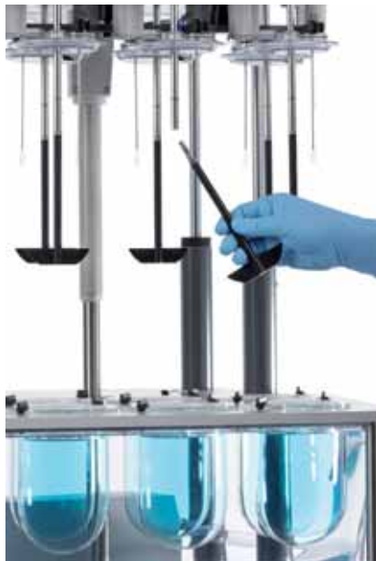
Upper shaft receptor and lower paddle piece
