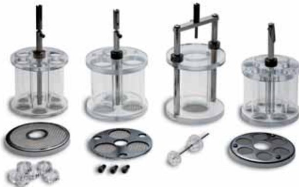
Agilent 100 accessories: (top row, left to right) 6-tube standard, 10-mesh basket; 3-tube, 10-mesh basket; 1-tube, 10-mesh basket; and 6-tube, 40-mesh basket; (bottom row, left to right) standard screen with fluted disks; 3-basket screen with screws, plunger; and 6-tube screen
