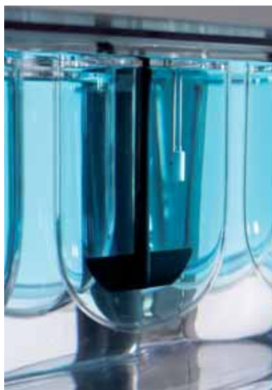
Non-resident sampling cannulas in a TruAlign vessel on the 708-DS.
