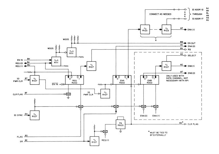
Figure 3–33 Multiplexer W104, Logic Diagram
