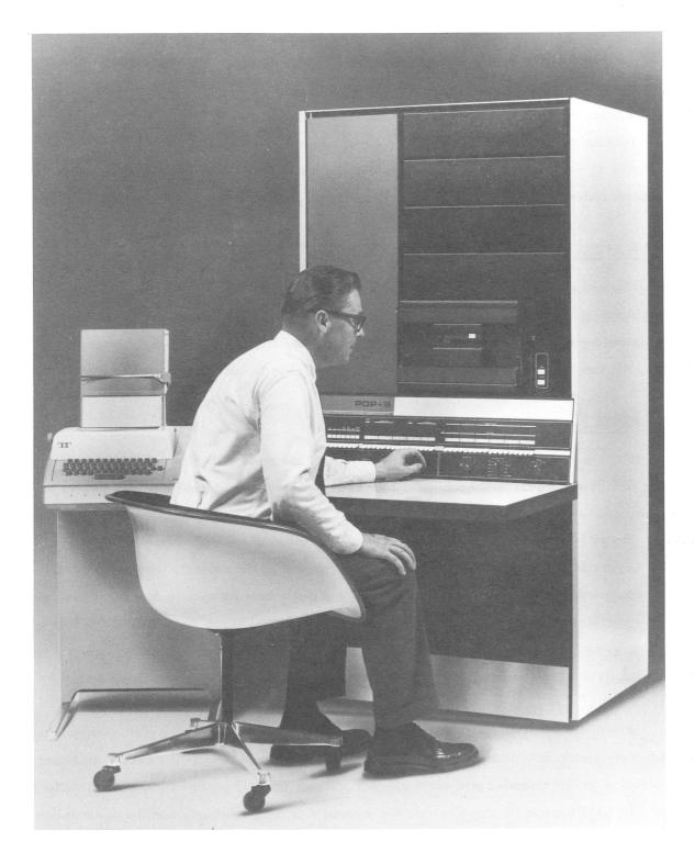
Figure 1–1 Programmed Data Processor PDP–9
