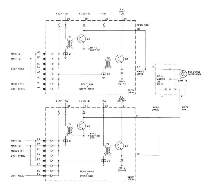
Figure 3-23 Digit Drive Selection, Bit 0, Line Y<sub>0</sub>
