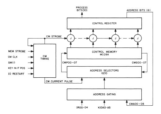
Figure 3-8 Control Memory System, Block Diagram
