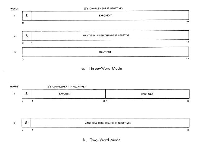
Figure 3-7 Floating Point Data Format
