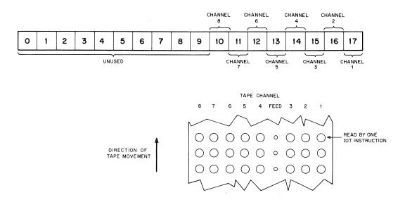
a. Tape Format and Reader Buffer Register Bit Assignments in Alphanumeric Mode
