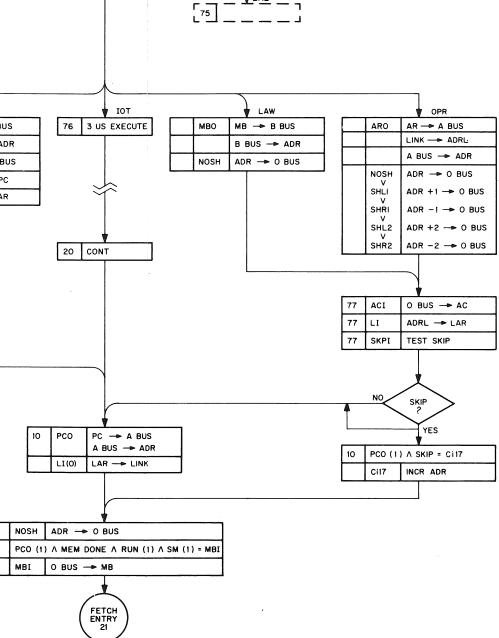
Figure 3-11 Fetch Cycle Flow, Sheet 2
