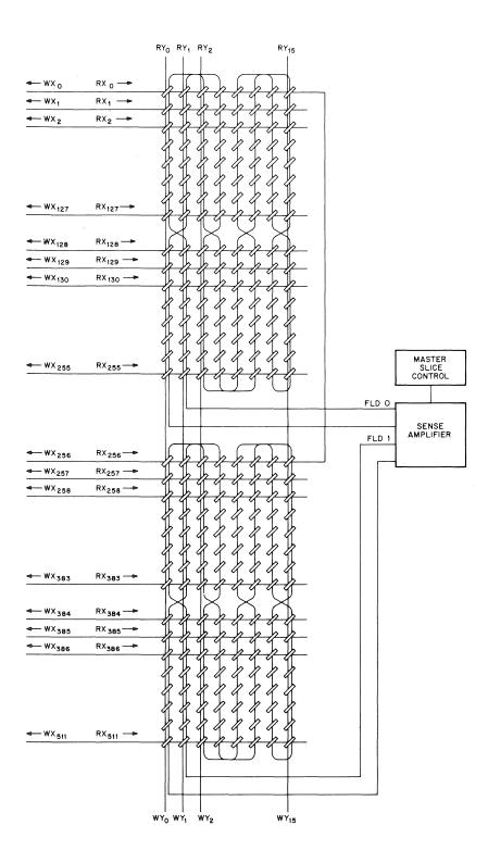
Figure 3-21 Core Wiring for One Bit Position
