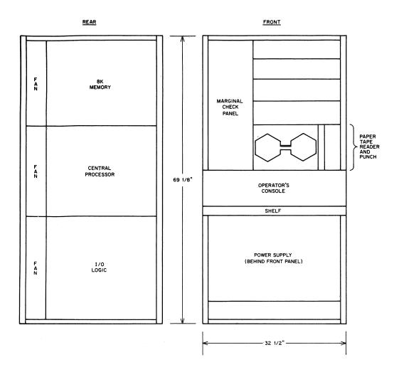
Figure 1-2 Basic PDP-9 Layout, Front and Rear
