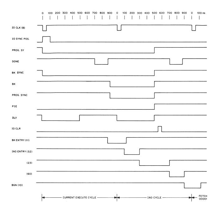
Figure 3-32 Program Interrupt Timing
