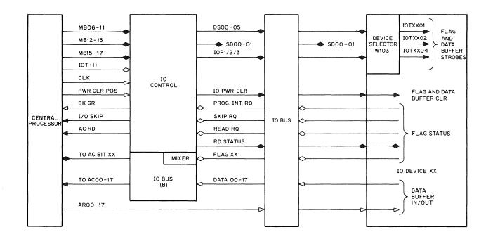
Figure 3-29 Program-Controlled I/O Interface
