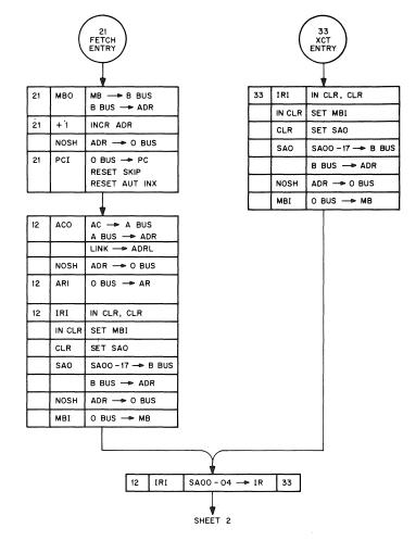
Figure 3-11 Fetch Cycle Flow, Sheet 1
