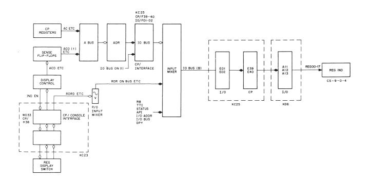
Figure 3-28 REGISTER DISPLAY Signal Paths
