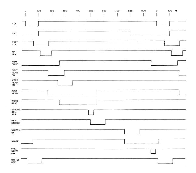
Figure 3-22 Core Memory Read/Write Timing
