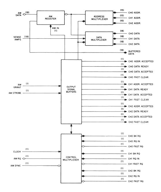
Figure 3-35 Adapter/Multiplexer DM09A, Block Diagram
