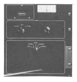
Figure 2-2 Marginal Check Panel and Maintenance Panel
