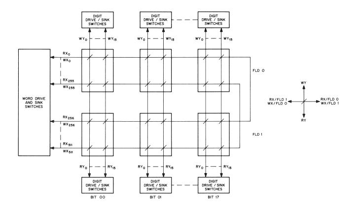
Figure 3–20 Planar Array Wiring
