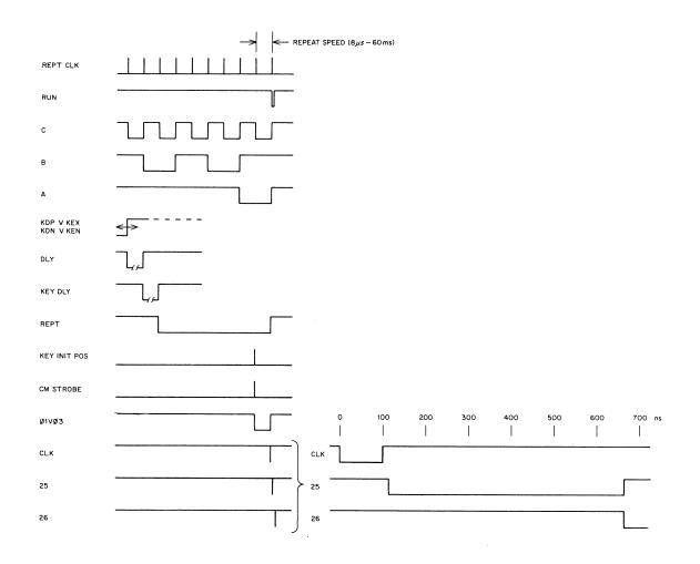
Figure 3-26 Initial Set-Up DEPOSIT or EXAMINE Timing
