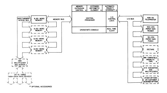
Figure 1-3 PDP-9 System Configuration, Block Diagram
