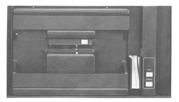
Figure 2-3 Paper Tape Reader/Punch PC09
