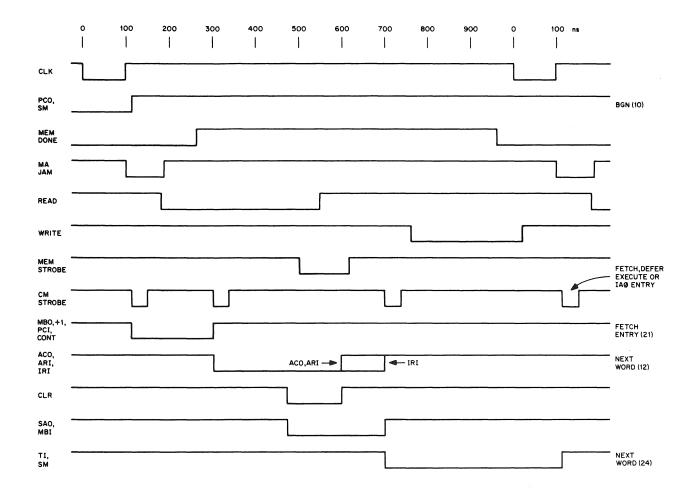
Figure 3-10 Fetch Cycle Timing
