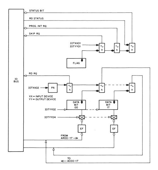
Figure 3-30 I/O Device Control Logic
