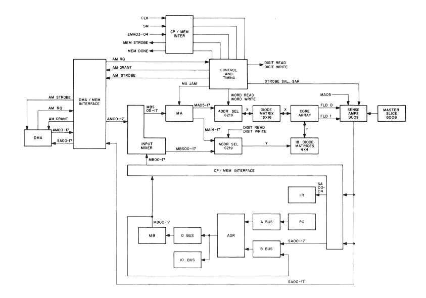
Figure 3–19 Core Memory System Block Diagram
