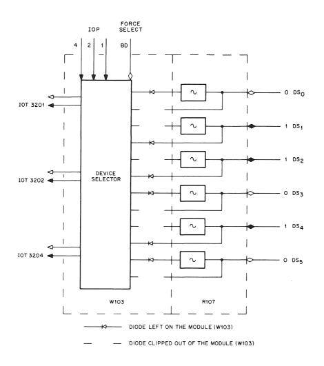
Figure 3-31 Device Selector W103, Schematic Diagram
