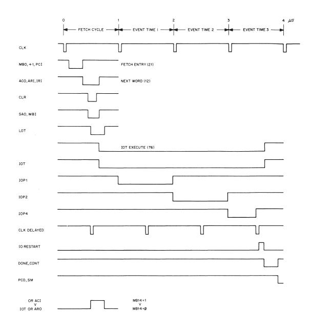
Figure 3-18 IOT Timing
