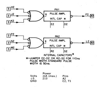
M602 Pulse Amplifier Simplified Diagram
