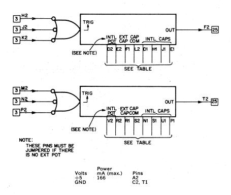
M302 Dual-Delay Multivibrator Simplified Diagram
