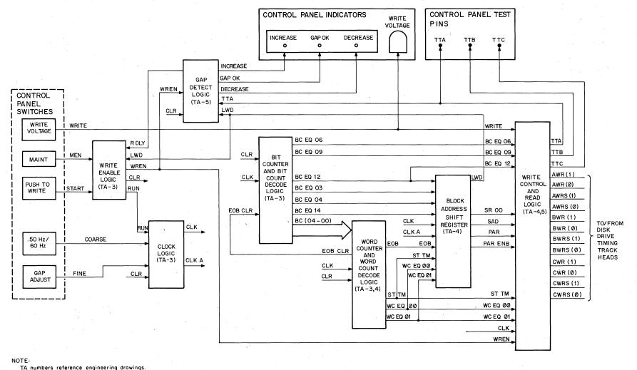
Figure 4-2 RS64-TA Functional Block Diagram
