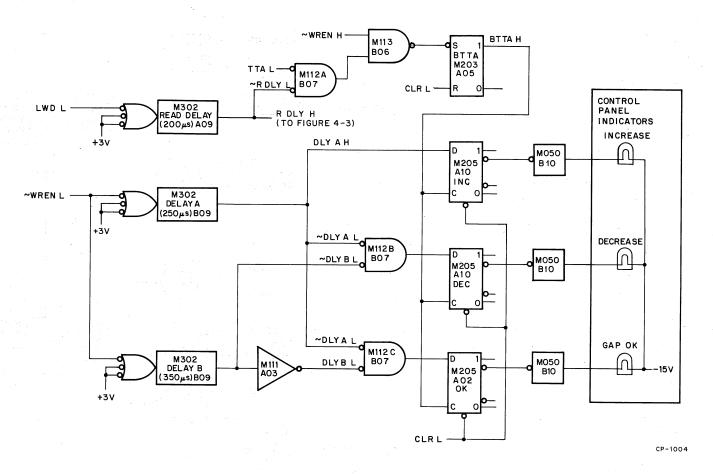
Figure 4-9 Gap Detect Logic Diagram
