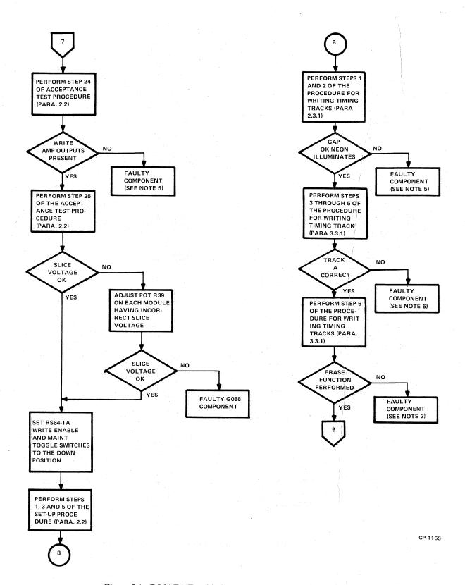
Figure 5-1 RS64-TA Troubleshooting Flow Diagram (Sheet 5 of 6)
