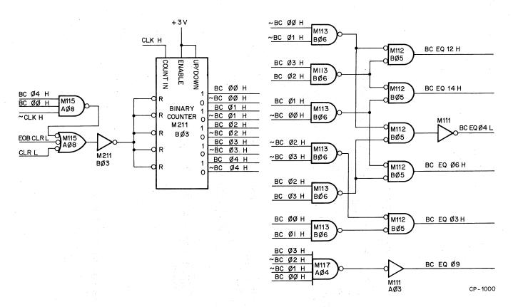
Figure 4-5 Bit Counter and Bit Count Decode Logic Diagram
