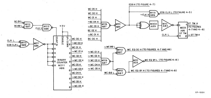
Figure 4-6 Word Counter and Word Count Decode Logic Diagram
