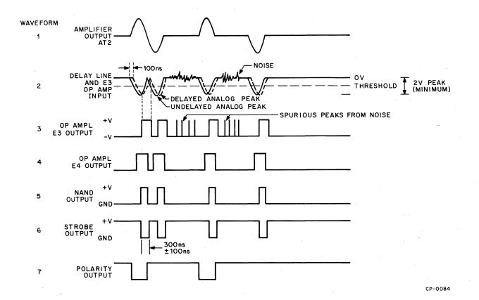
G088 Read Amplifier-Peak Detector Waveforms
