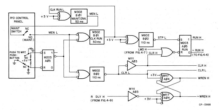
Figure 4-3 Write Enable Logic Diagram
