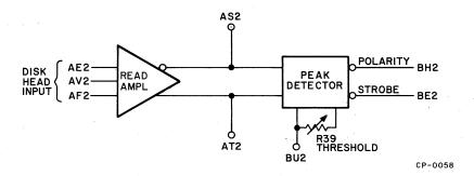
G088 Read Amplifier-Peak Detector Simplified Diagram
