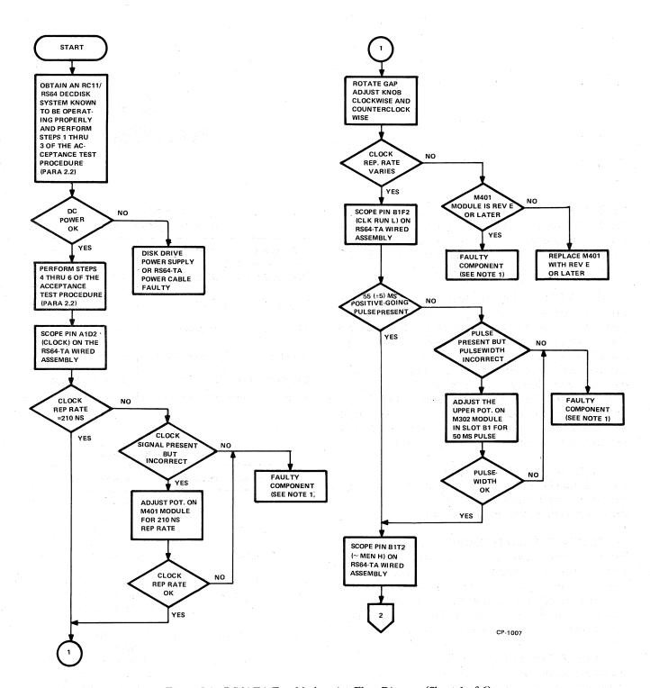
Figure 5-1 RS64-TA Troubleshooting Flow Diagram (Sheet 1 of 6)
