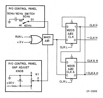
Figure 4-4 Clock Logic Diagram
