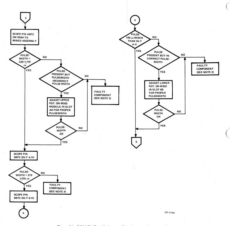
Figure 5-1 RS64-TA Troubleshooting Flow Diagram (Sheet 3 of 6)
