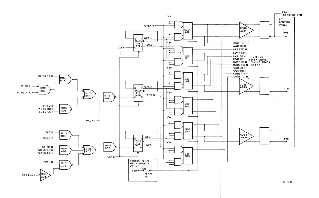
Figure 4-8 Write Control and Read Logic Diagram
