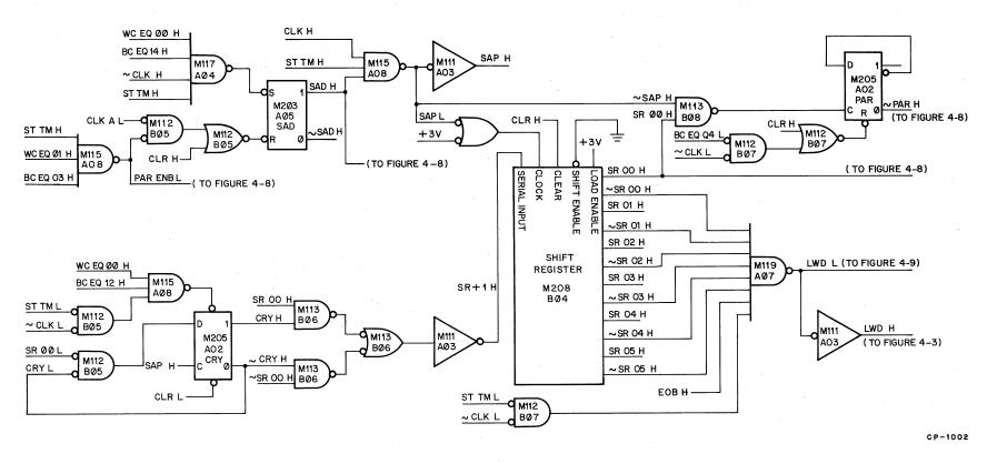
Figure 4-7 Block Address Shift Register Logic Diagram
