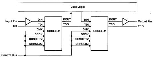
Figure 9. Boundary Register Using UBCELL2
