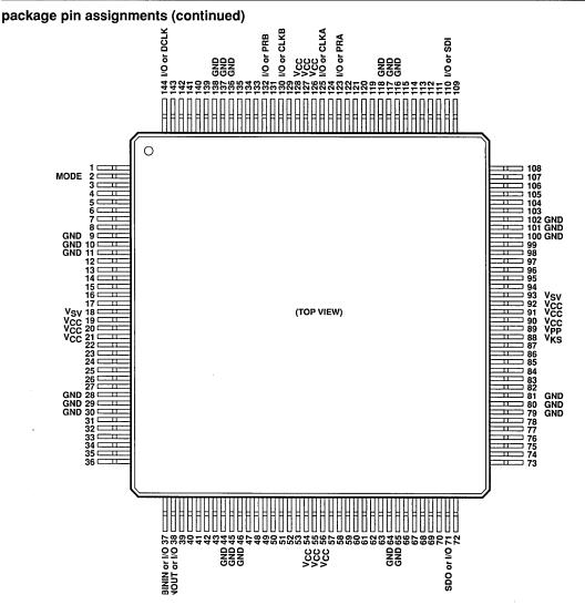
NOTES: A. All pins marked GND are ground connections and must be connected to circuit ground.
