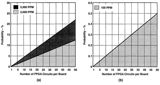
Figure 5. Defect Probability vs PPM Level
