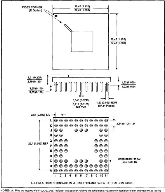
NOTES: A. Pins are located within 0,13 (0.005) radius of true position relative to each other at maximum material condition and within 0,381 (0.051) radius relative to the center of the ceramic.
