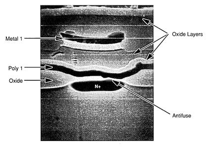
Figure 5–1. Antifuse SEM Cross-Section
