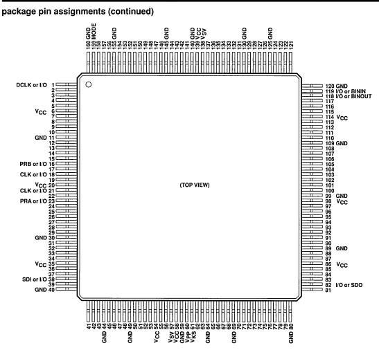
NOTES: A. Aii pins marked GND are ground connections and must be connected to circuit ground.
