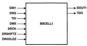
Figure 10. Bidirectional Boundary Cell 1
