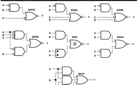
Module Count = 1 (unless otherwise noted) (2) Indicates Module Count = 2 A Indicates extra delay input
