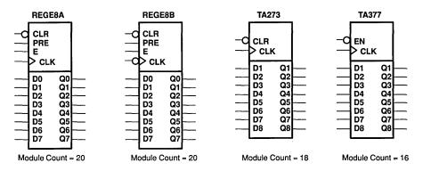
Figure 28. Octal D-Type Flip-Flops and Registers
