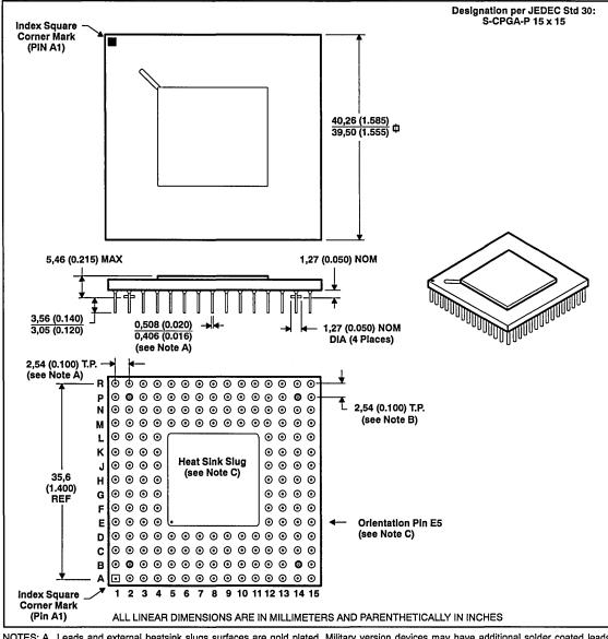
NOTES: A. Leads and external heatsink slugs surfaces are gold plated. Military version devices may have additional solder coated leads. Diagrams do not include the solder finish where applicable.
