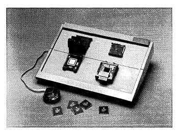
Figure 3–4. Activator 2 Programmer
