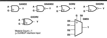
Figure 33. Clock Buffer (CLKBUF) Interface
