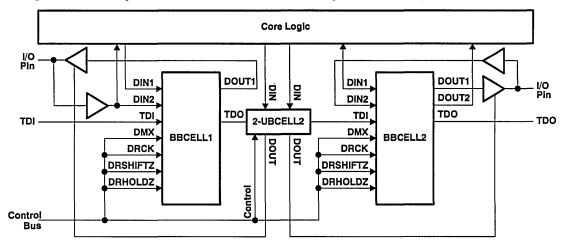
Figure 11. Boundary Register Using BBCELL1
