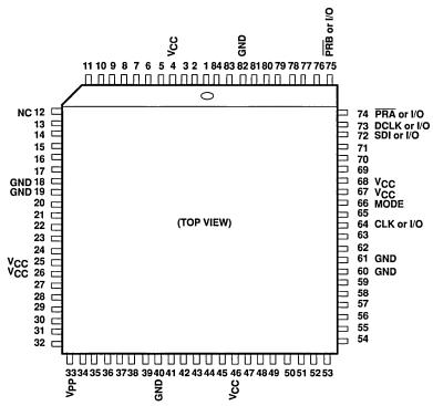
NOTES: A. All pins marked GND are ground connections and must be connected to circuit ground.
