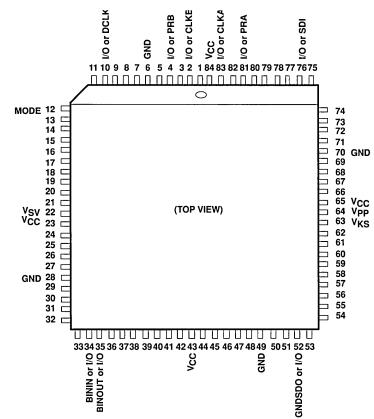
NOTES: A. All pins marked GND are ground connections and must be connected to circuit ground.
