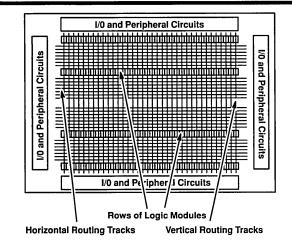
Figure 1. Diagram of TPC14 Series Architecture
