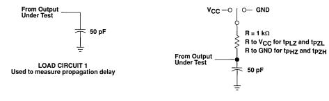
LOAD CIRCUIT 2 Used to measure rising/falling edges
