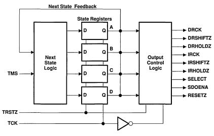
Figure 2. TAP Block Diagram
