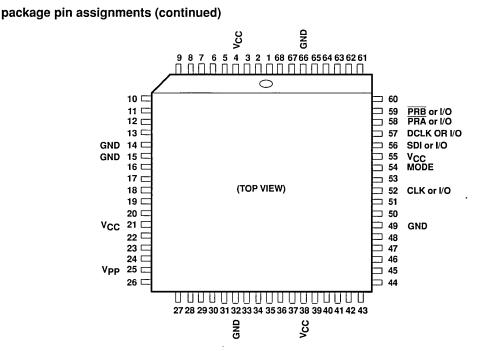
NOTES: A. All pins marked GND are ground connections and must be connected to circuit ground.
