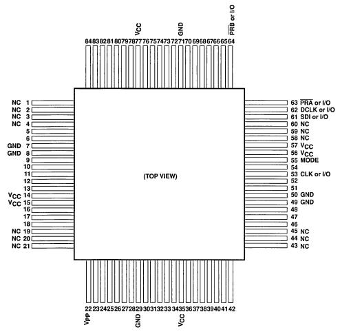
NOTES: A. All pins marked GND are ground connections and must be connected to circuit ground.
