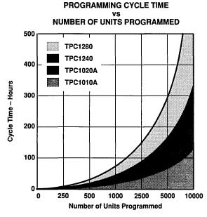
Figure 2. FPGA Programming Cycle Time
