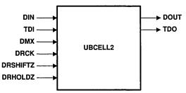
Figure 8. Unidirectional Boundary Cell 2
