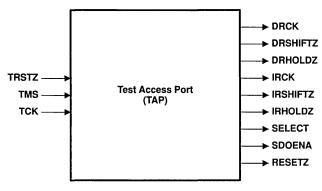
Figure 1. Test Access Port (TAP)
