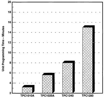
Figure 1. FPGA Per Unit Programming Time
