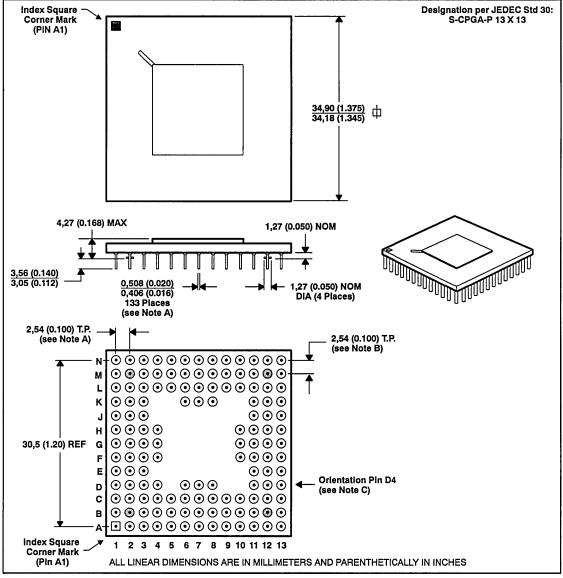
NOTES: A. The lead finish is solder coated. The dimensions do not include the solder finish.
