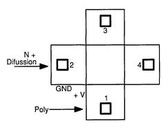
Test devices were stressed by forcing a constant 5 mA current from polysilicon to N+ through the antifuse at 250°C. Note that this stress is far greater than a programmed antifuse would see in a device under normal operating conditions. Because the antifuse is used to connect two networks together, there is usually no voltage across it and hence no current passes through. A voltage will appear across the antifuse only momentarily while a network switches from low-to-high or high-to-low.
