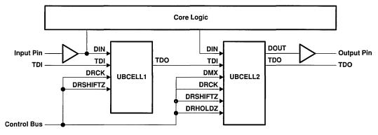
Figure 7. Boundary Register Using UBCELL1
