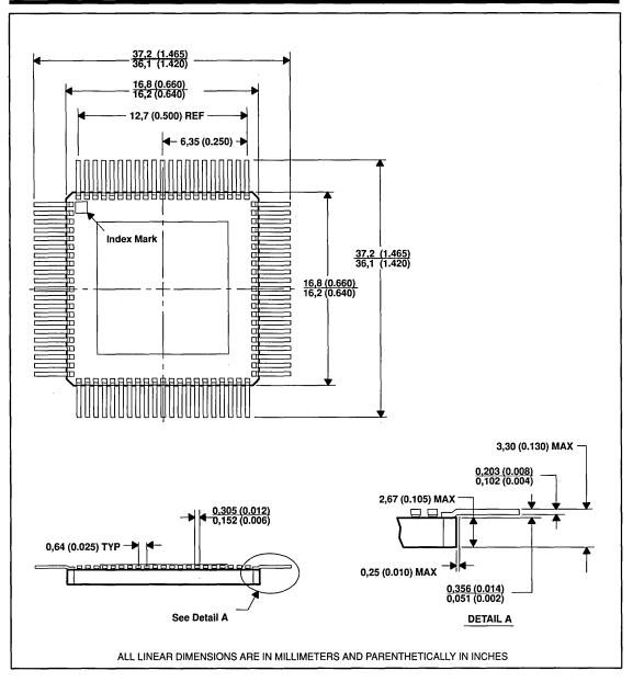
Figure 49. 84-Pin Ceramic Quad Flat Package
