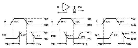
Figure 5. Symbols, Test Loads, and Waveforms
