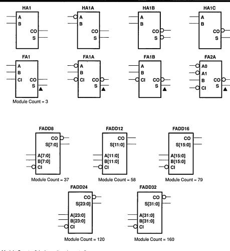
Module Count = 2 (unless otherwise noted) ▲ Indicates two logic module delay path
