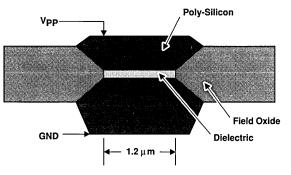
Metal routing tracks run horizontally and vertically over the die, with an antifuse at each intersection. The unprogrammed resistance of the antifuse is greater than 100 M $\Omega$  and the programmed resistance is approximately 500  $\Omega$ .
