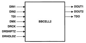
Figure 12. Bidirectional Boundary Cell 2
