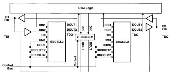
Figure 13. Boundary Register Using BBCELL2
