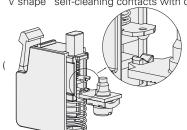
This shape, thanks to its quadruple support, allows to reduce the probability of contact wrong switching. Furthermore it highly improves the contacts reliability in case of dust registered patent).
