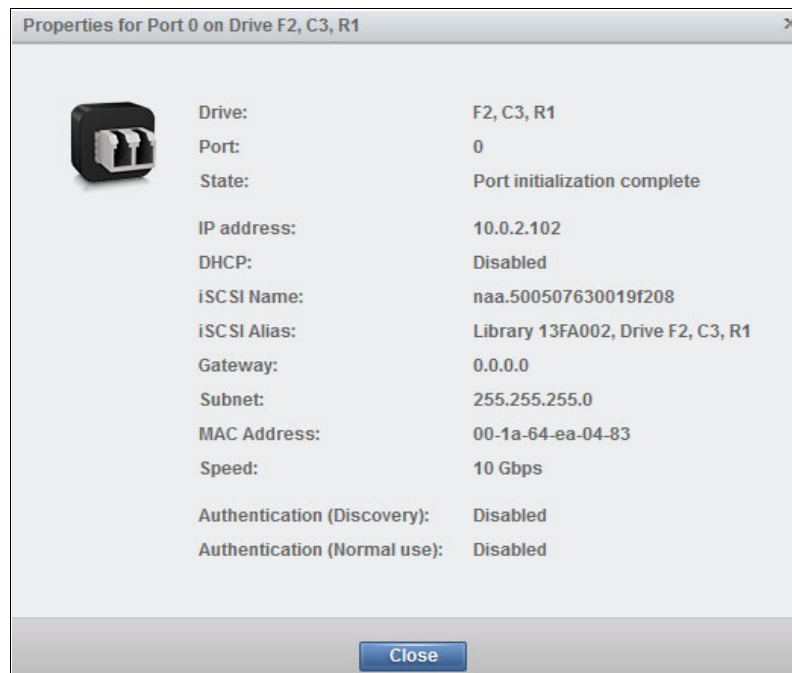
Figure 4-116 Ethernet port properties
