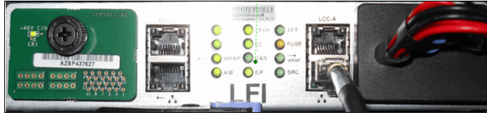
Figure 1-40 Library frame interconnect (LFI)
