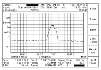
Fig. 8-19 Measurement menu after pressing the Exec Zoom softkey
