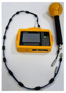
Fig. 5-4 Connecting the SRM-3000 and antenna with a cable
