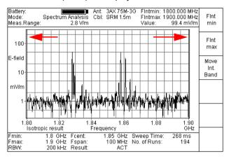
Fig. 8-27 Integrating the level value over a frequency band
