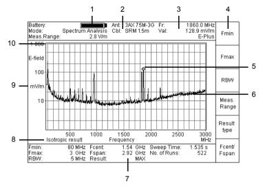
Fig. 8-2 Measurement menu for "Spectrum Analysis" mode
