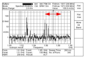
Fig. 8-29 Upper limit of frequency band
