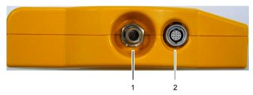
Fig. 6-3 Antenna and control cable connector sockets
