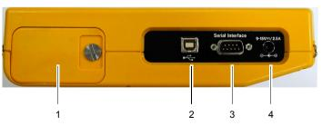
Fig. 6-4 Battery holder and external connectors
