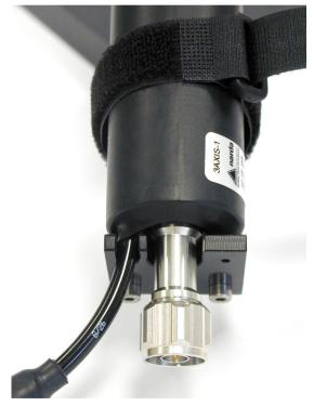
Fig. 5-7 Cable and N connector in guide groove
