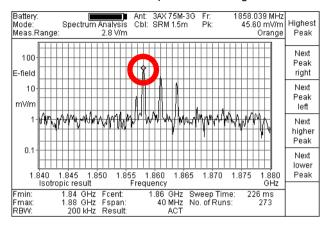
Fig. 8-21 Moving the marker with the Highest Peak softkey
