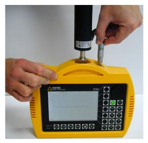
5. Press the control cable plug into the connector using the locking sleeve until the plug lock clicks into place.
