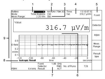
Fig. 10-2 "Time Analysis" mode measurement menu
