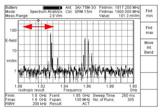
Fig. 8-28 Lower limit of frequency band
