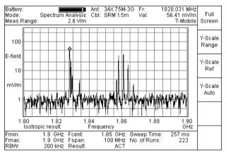
Fig. 8-9 Softkeys for selecting the display mode and scaling
