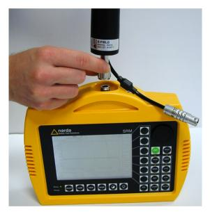
Fig. 5-2 Connecting up the N connectors
