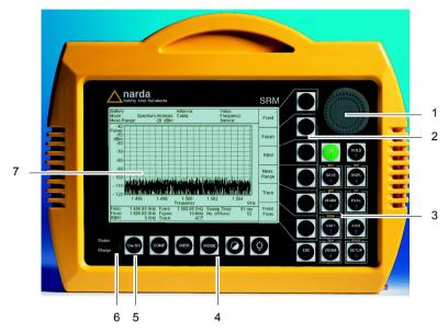
Fig. 6-1 Display and control elements
