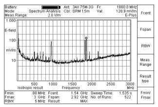
Fig. 11-1 "Spectrum Analysis" mode (Isotropic result)
