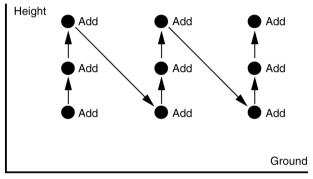
Fig. 12-2 Example of discrete measurement recording of three separate values at each of three positions in a room
