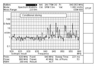
Fig. 13-5 Display during automatic storage
