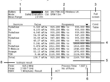
Fig. 7-2 Measurement menu for "Safety Evaluation" mode
