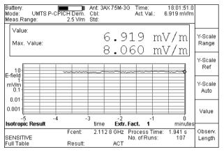
Fig. 9-6 Mixed display mode (numerical display with graphical display versus time)
