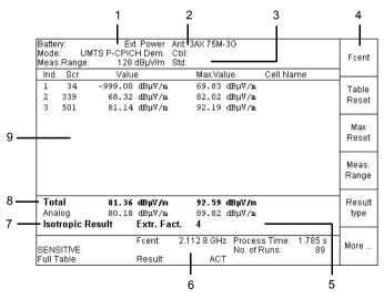
Fig. 9-2 Measurement menu for "UMTS P-CPICH Demodulation" mode
