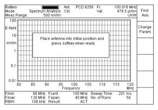
Fig. 11-6 "Spectrum Analysis" mode; isotropic measurement with a single axis antenna
