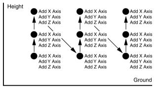
Fig. 12-3 Three separate measurements are needed at each point if a single axis antenna is used
