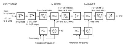
Fig. B-1 Block circuit diagram of RF module
