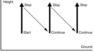
Fig. 12-1 Example of continuous measurement recording at three positions in a room
