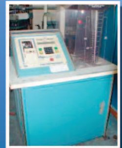
KENCO IONIC CONTAMINATION SYSTEM;MODEL #600; 18 X 18 TEST CELL Price: $900 Search: ZM-453F
