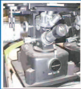
UNITRON METALLURGICAL MICROSCOPE;#MeC 10176; 6"X6" STAGE;40, 5, 10 POWER OBJECTIVES;1 X 1.5" MOVEMENT Price: $1750 Search: ZM-8230
