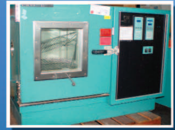
Thermotron Model SM-3.5S Temperature/Humidity Chamber Internal: 16"(w) x20"(d) x18"(h) Temp: -20C to +95C Humidity: 20% to 95%RH Price: Search: CH-580F
