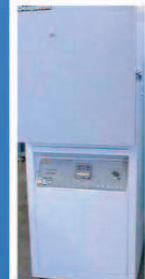
Despatch 16207 Temp Chamber Internal: 20"(w) x 24"(d) x 25"(h) Temp: -20C to +177C Price: $5900 Search: CT-9476
