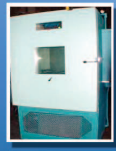
Tenney Temp/Humidity Chamber Model TH-27 Internal: 38"(w) x 26"(d) x 48"(h) Temp: -10C to +93C Humidity: 20% to 95%RH Price: $9800 Search: CH-533F
