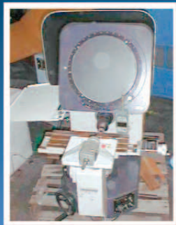
MITUTOYO;#PH-350; 15" X 6" STAGE; DIGITAL GAUGES 20X LENS;14" SCREEN Price: $3500 Search: ZM-345A
