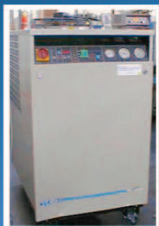
MTA WATER CHILLER; MODEL #TAE-0051;460V;3PH; 14 AMPSAIR-COOLED;NEVER USED Price: $6300 Search: ZM-407C
