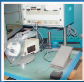
HUGHES PARALELL GAP WELDER; MODEL #MCW-550-CO2;120V; COMP. W/MICROWELD VTA 96 HD; B & L STEREOZOOM 4 W/FOOT PEDAL; GOAL POST ASSEMBLY
