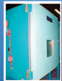
Tenney AGREE Chamber Model AG-40 Internal: 40"(w) x 40"(d) x 36"(h) Temp: -70C to +177C Price: $26,000 Search: CZ-7355
