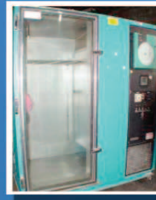
Bemco Model FW30-2/100C Temp/Humidity Chamber Temp: -18C to +94C Price: $10,500 Search: CH-702F
