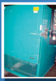
Bemco F-100-350 Temperature Chamber Internal: 36"x36"x36" Temp: -65C to +170C Price: $9800 Search: CT-635F
