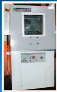
Despatch Temp/Humidity Chamber Model 16519M Internal: 34(w) x 30"(d) x 32"(h) Temp: -20C to +170C Humidity: 20% to 95%RH Price: $10,200 Search: CH-484A
