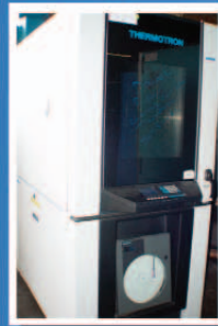
Thermotron Model SE-300-2-2 Temperature Chamber Volume: 10.2 cu. ft. Temp: -73C to +200C Price: Please Call Price: Best Price - Pse Call.
