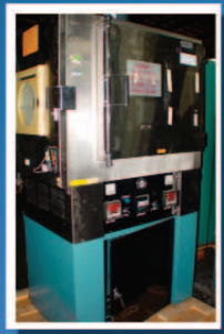
Blue M Model AC-7602 Temp/Humidity Chamber Internal: 25"(w) x 20"(d) x 19"(h) Temp: 12C Above Ambient to 93C Price: $6600 Search: CH-701F
