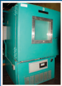
Thermotron Model SM-32C Temperature/Humidity Chamber Internal: 38"x38"x38 Temp: -70C to +170C Price: $13,500 Search: CH-840F
