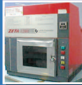
LOCTITE UV CURING SYSTEM; MODEL #ZETA7200;9X8X7;120V;20 AMPS; P.#983120/UVA&UVB REGIONS; PART SIZE 5X6;300W Price: $4300 Search: ZM-956A
