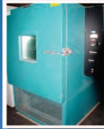
Bemco F-100/350-16 Temperature Chamber Internal: 30"(w) x 28"(d) x 30"(h) Temp: -70C to +170C Price: $9800 Search: CT-859F
