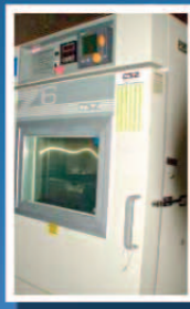
CSZ Z16-2-2-H-W/C Temperature Chamber Internal: 30"x30"x30" Temp: -70C to +170C Price: $9500 Search: CT-507F
