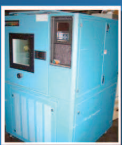
Envirotronic Temp/Humidity Chamber Model SH8 Internal: 24"x24"x24" Temp: -30C to +177C Humidity: 20% to 95%RH Price: $8400 Search: CH-583F
