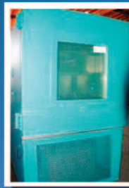
Tenney Model TR-40 Temp/Humidity Chamber Internal: 40 cu. ft. Temp: -25C to +170C Humidity: 20% to 95%RH Price: $13,500 Search: CH-401F
