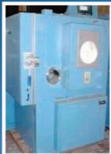
Thermotron Remote Cooling System Model PRCH3-3 Temp: -73C to +177C Price: $7500 Search: CZ-6255
