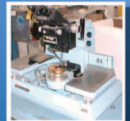
WENTWORTH PROBE STATION; MODEL #0-037-1112;4" CHUCK B & L MICROZOOM W/ISOLATION TABLE Price: $4500 Search: ZM-2600
