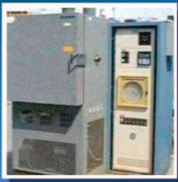
Blue M VRC08-PW Temperature Chamber Fast Ramping Internal: 24"x24"x24" Temp: -70C to +170C Price: $10,400 Search: CT-497C
