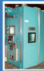
Qualmark HALT Chamber Model OVS-3 Internal: 38"(w) x 43"(d) x 36"(h) Temp: -70C to +90C Price: $29000 - Sold As Is Search: CZ-656F
