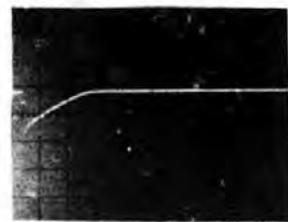
10 .2 V/cm .2 μsec/cm dc coupled - slope
