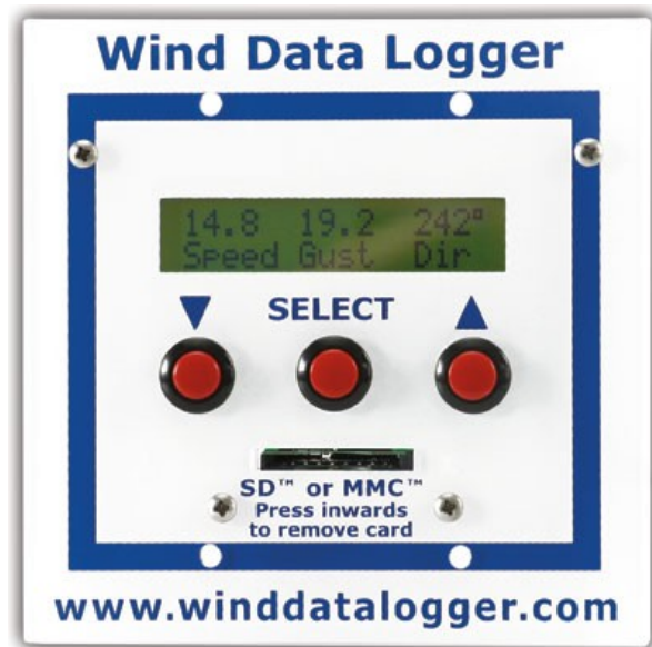
Figure 8. Formatting the memory card. Memory card must be formatted in either FAT12 or FAT16. FAT 32 does not work.
