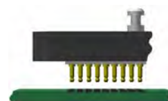
Raised SMT type (lifts socket above close-by components)
