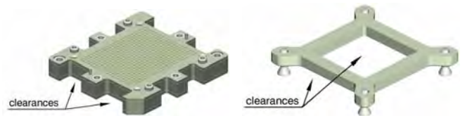
Socket body with clearances
