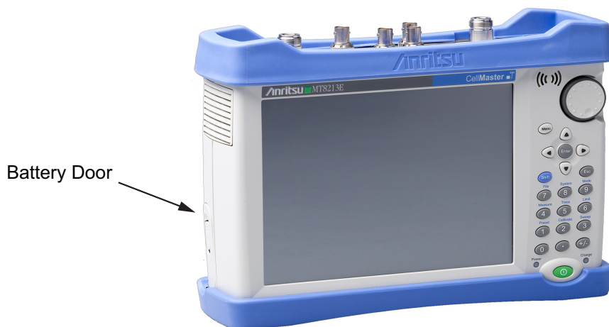
Figure 6-1. Battery Access Door Location
