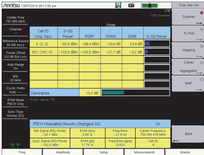
Figure 5-11. Over-the-Air Scanner Measurements
